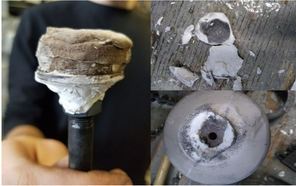
Figure A.13: Failed stopper rod made of high-temperature Kaowool ceramic blanket
