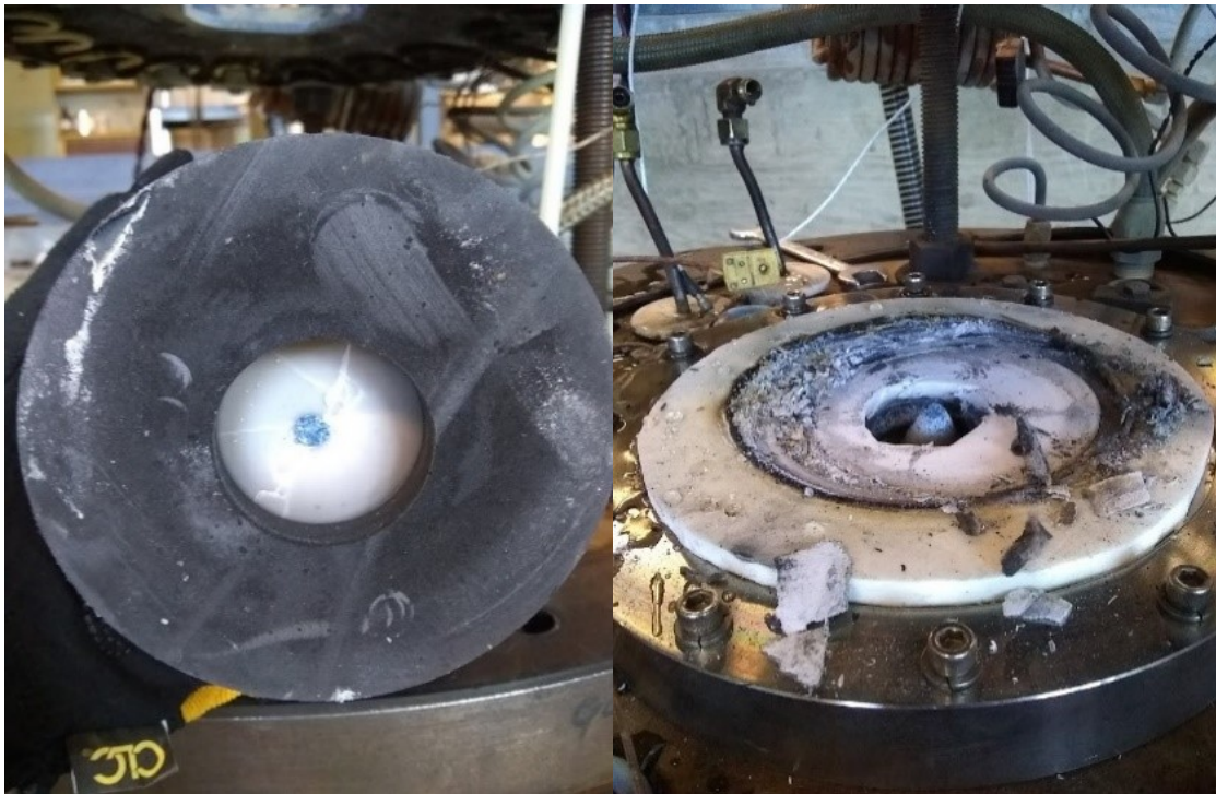
Figure A.15: Failed stopper rod made of cast Ceramacast 510
