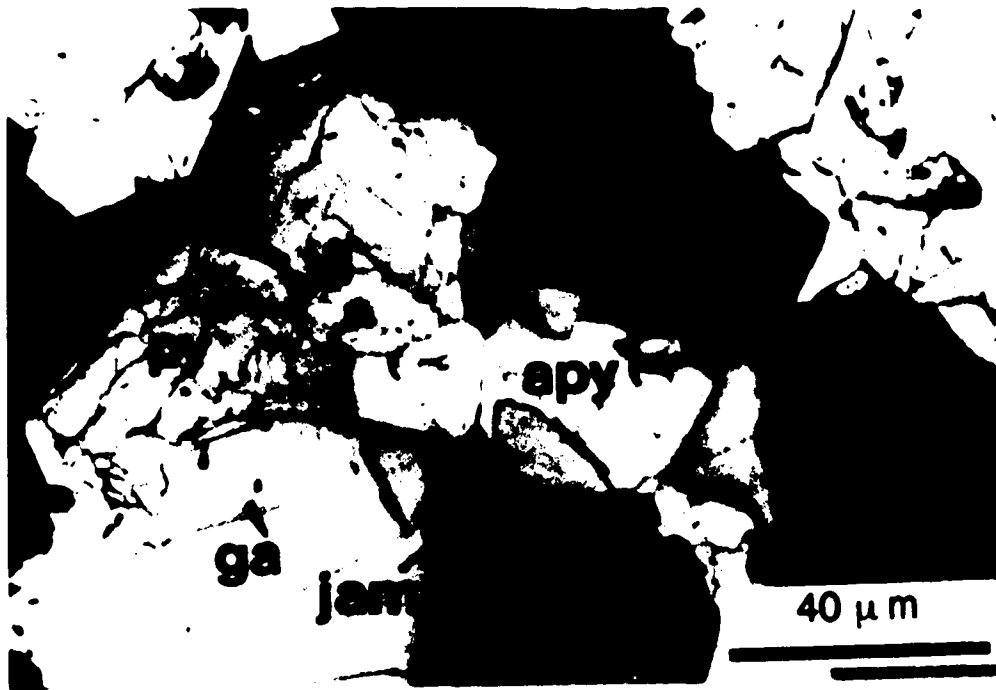
Figure 4-13. Polished section, MINTO 01. Plane polarized light. Typical sulphide assemblage in Minto ore.
