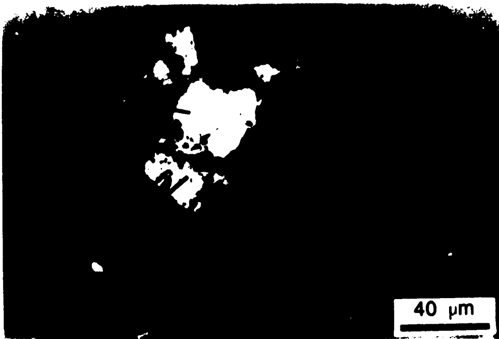
Figure 4-8. Polished section, HOW 08. Plane polarized light. Gold replacing stibnite.
