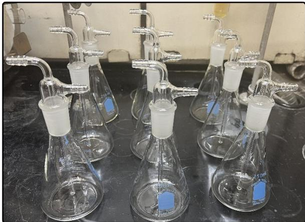
**Figure 7.2.** The HCl trap used to capture gaseous HCl by bubbling the emissions through 2M NaOH solution.
