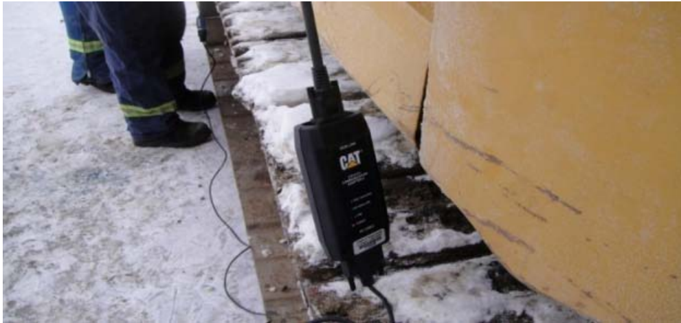
Figure 19: The CAT data logger
