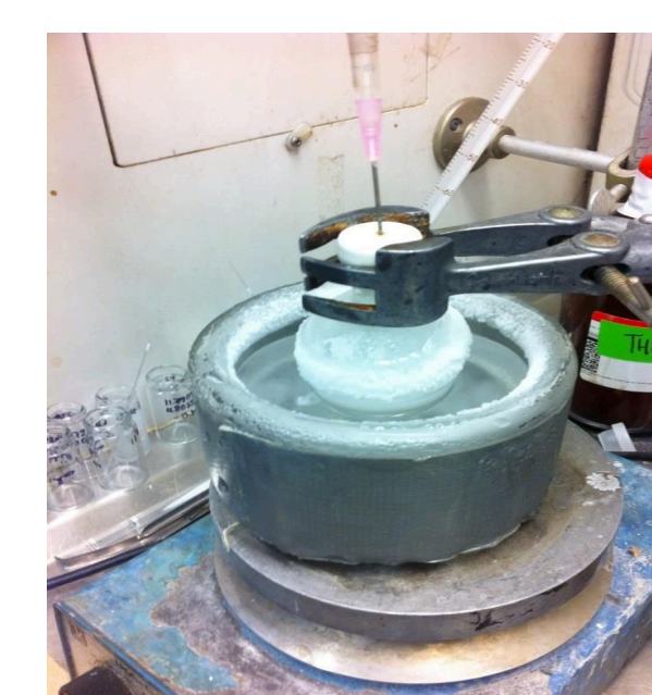
Figure 5: Swern Oxidation: CO 2 Cl 2 , DMSO and DCM at -78°C
