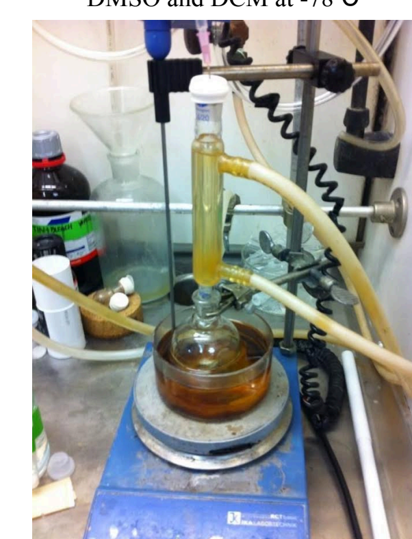
Figure 7: Reaction under argon at 165°C,
