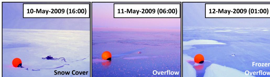
Figure 2-18 Pictures from the time-lapse camera at ST-2009 in May 2009 showing the variation in the floating sea ice overflow depth.
