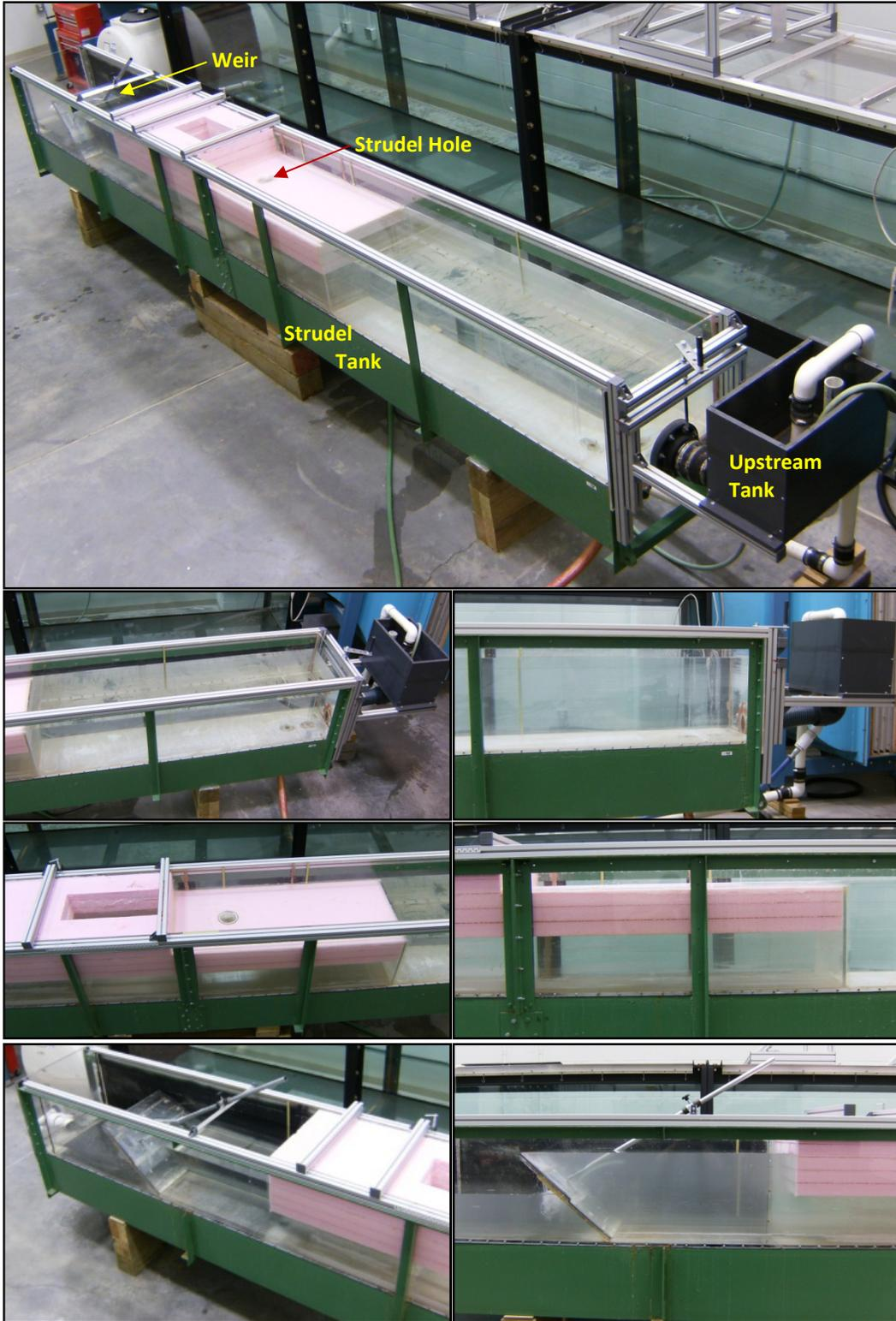
Figure 3-7 Picture of the *Upstream Tank* and of the *Strudel Tank*. The flow direction is from right to left.
