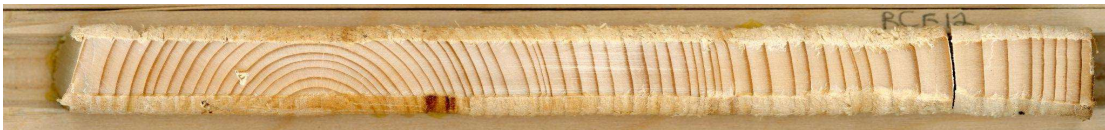
Figure 3. Example of a core sampled from a wooden cabin as part of this project.
