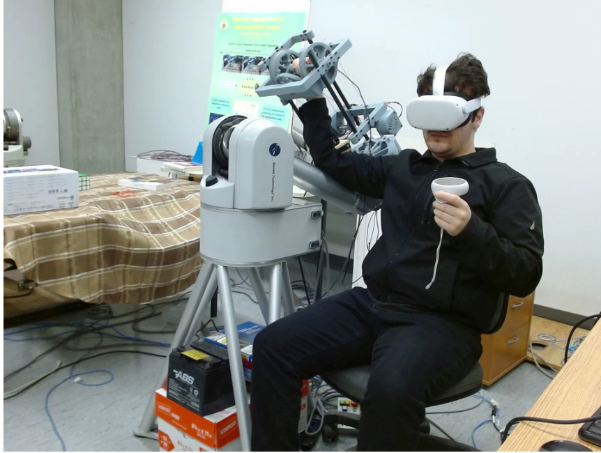
Figure 3.5: The configuration for the operator with the leader robot arm and head-mounted display.
