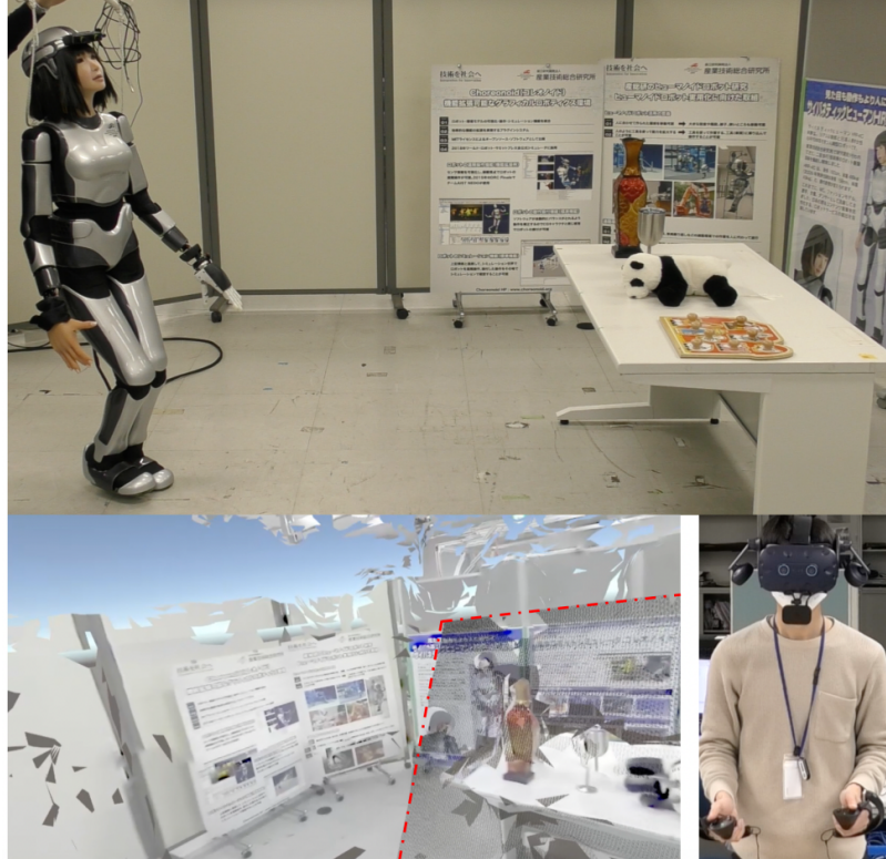
Figure 2.21: Immersive display can induce motion sickness, the decoupled view helps to reduce motion sickness caused by the latency [124].
