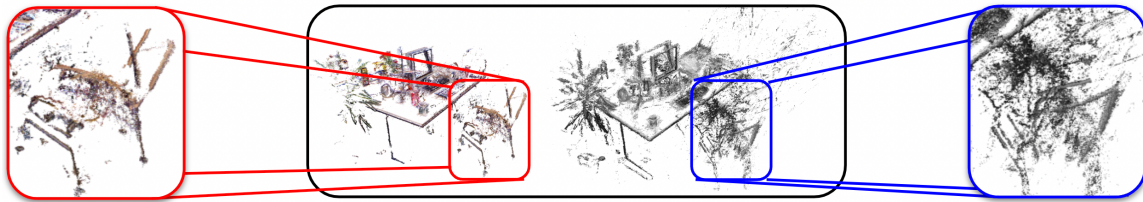
Figure 2.10: Compared to LSD-SLAM, ORB-SLAM semi-dense module is more accurate due to getting points along epipolar lines.
