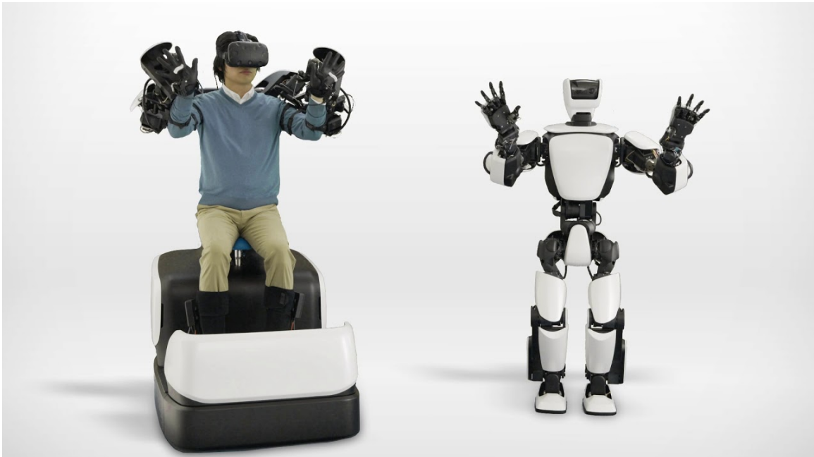
Figure 2.20: Immersive display helps the operator to control the view of the remote environment [113].
