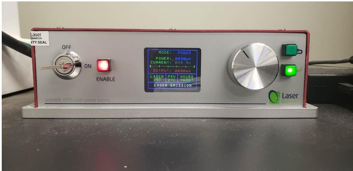
**Figure 2.4.** Laser system control module. The red “ENABLE” light indicates the laser is on.
