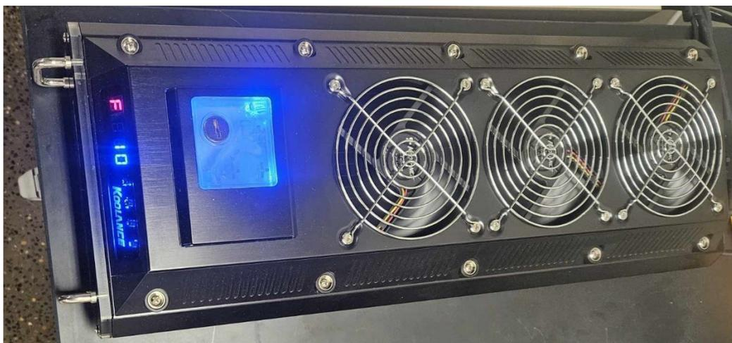
**Figure 2.8.** A picture of EX2-755\_KOOLANCE superior liquid cooling system. F stands for the Fan mode.
