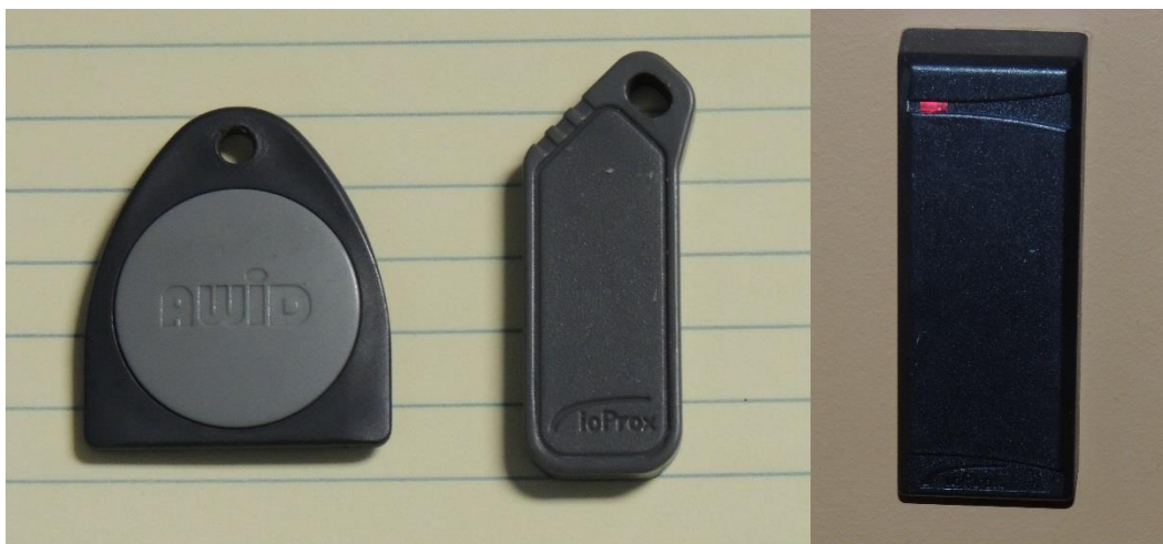
Figure 7: Samples of Access Control Devices (Security Fobs and Reader)
