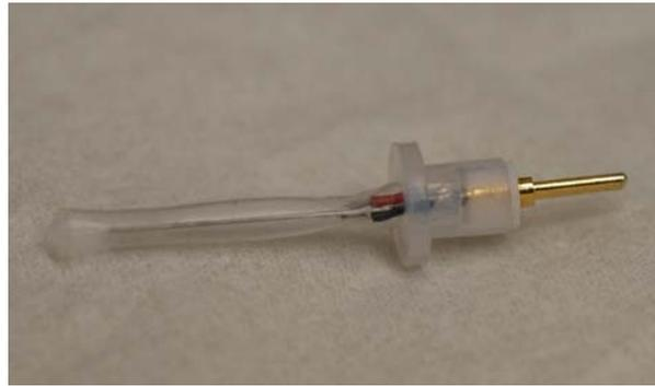
**Fig. 9-4** Photograph of bimorph force sensor used in the experiments.
