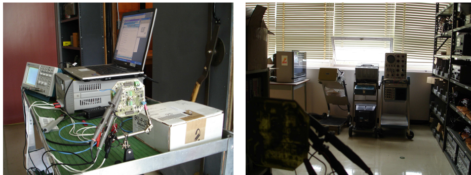
Figure 5.6: Ambient light to voltage output measurement environment – light level controlled by blinds and detector distance from window.
