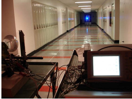
Figure 5.21 Distance measurement – receiver at 30 meters from light source.
