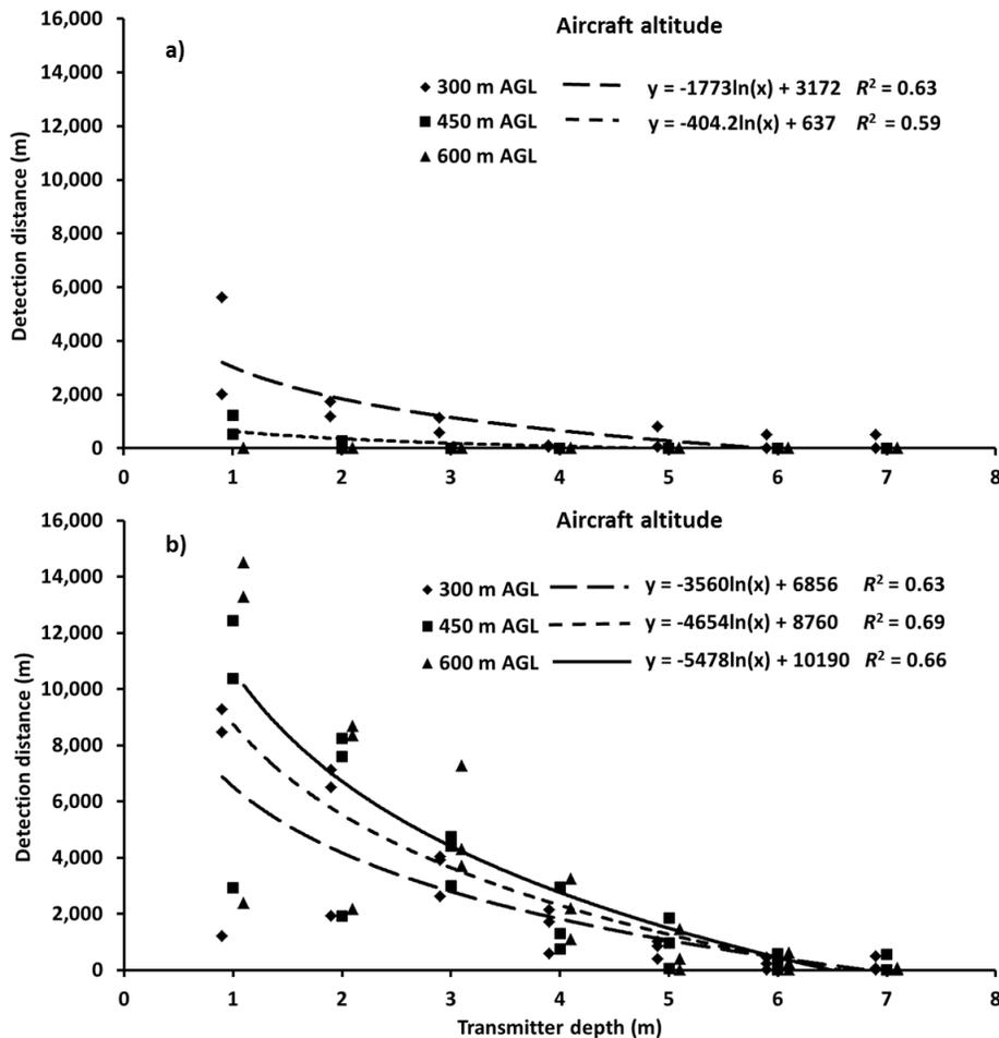
Figure 4.1. Detection distance at different depths and receiver altitudes for small type (a) and large type (b) radio transmitters in the North Saskatchewan River, Alberta.
