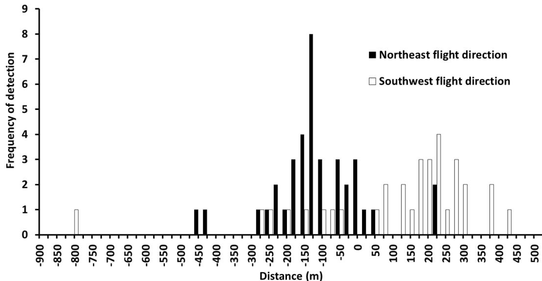
Figure 4.2. Estimated positional location of two transmitter types, depths and receiver altitudes for aerial surveys flown in either a northeast or southwest direction in the North Saskatchewan River, Alberta. Negative values represent estimated locations that are to the northeast of the actual location and positive values are estimated locations to the southwest.
