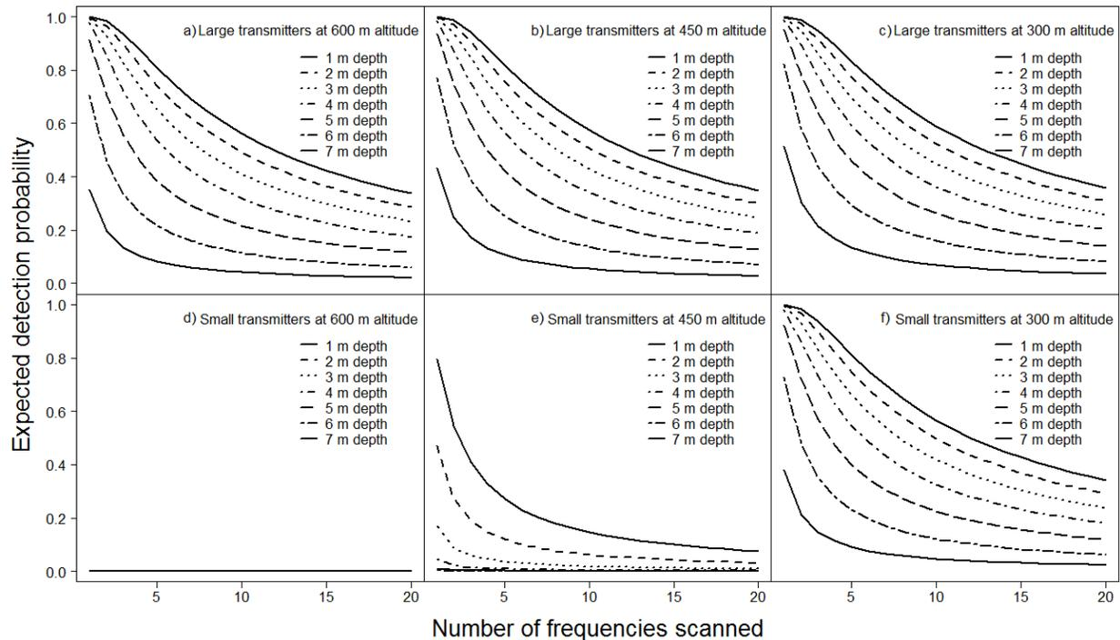
Figure 4.4. Expected detection probability versus number of frequencies scanned for the two transmitter types at different depths and receiver altitudes in the North Saskatchewan River, Alberta.
