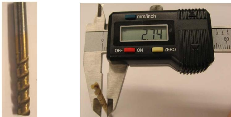
Figure 4-2: The photos of a steel drill bit (left) and its width (right).
