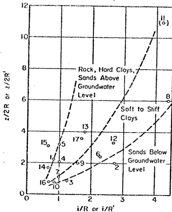
FIG. 5B Relation Between Width of Settlement Trough, as Represented by  $i/R$ , and Dimensionless Depth of Tunnel,  $z/2R$ , for Various Tunnels in Different Materials
