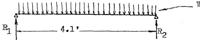
$$w_z = (K_0 \gamma z) \frac{1}{2} = 1(5260) \frac{1}{2} = 2630 \text{ \#/ft of lagging} = 219 \text{ \#/in lagging}$$
