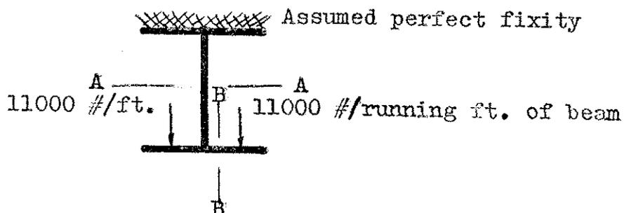
Considering section A-A under symmetrical loading
