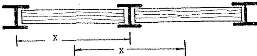
Each stiffening rib has transferred to it via the lagging a load dependent on the spacing of the ribs.
