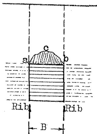
Terzaghi (1943) has outlined the theory of arching in soils. Laboratory investigations have shown that the pressure on a yielding strip such as a-b is almost independent of the state of stress existing in the soil at a height of more than 2B to 3B above the top of the strip.
