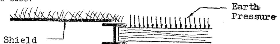
This case may arise during tunnelling, i.e. where the stiffening ribs have been left unsupported and there is only an applied load from the lagging on one side.
