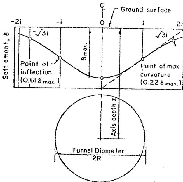
Ratio  $\frac{i}{R}$  is function of  $\frac{z}{2R}$  and soil conditions
