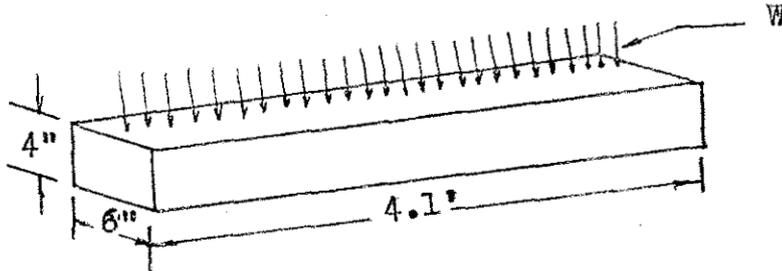
First consider the long-term condition where no axial loads are applied to the lagging from the forward jacking of the shield.
