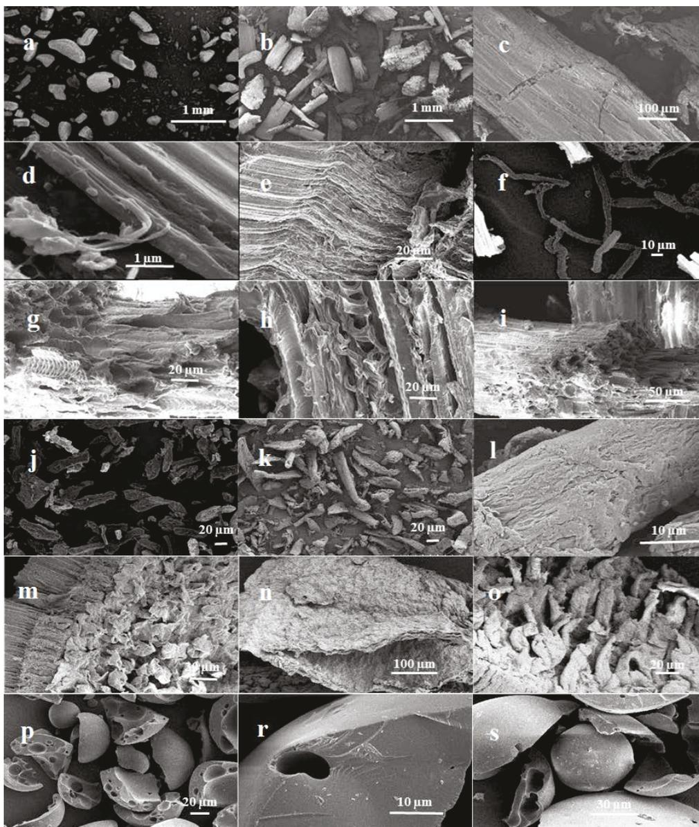
**Figure 4-5.** Scanning electron microscopy (SEM) images of (a) untreated lupin hull, (b,c) untreated canola straw, (d-f) NaOH treated lupin hull, (g-i) NaOH treated canola straw, (j) NaOH-ASC treated lupin hull, (k,l) NaOH-ASC treated canola straw at the optimized conditions (NaOH: 15%/99 °C/6h, and ASC: 1.7%/75 °C/6h), (m-o) lignin from lupin hull, and (p-s) lignin from canola straw after NaOH treatment (15%/99 °C/6h).
