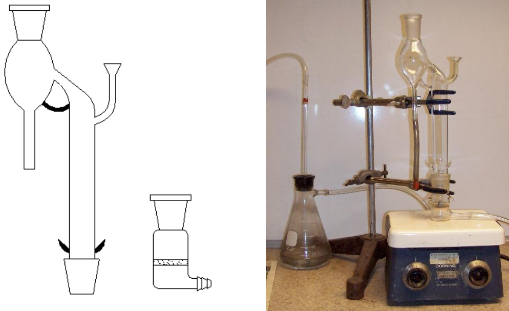
Figure 25: "Siwek" type micro-scale flotation tube
