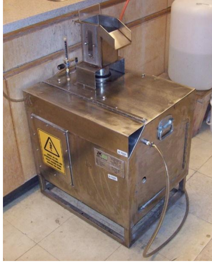
Figure 26: JK Tech bottom drive flotation machine and 1.5 L cell
