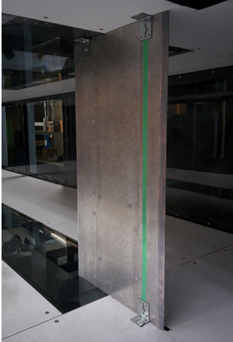
Figure 3.2: Photograph of the blunt body model mounted within the test section. The green strip near the leading edge of the model represents the location of the trip wire.
