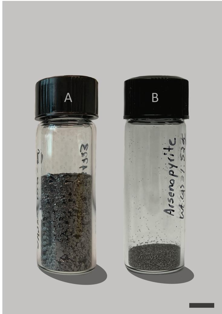
**Figure A9.** Sample vials containing equal mass proportions (1.5 g) of pure graphite (A) and arsenopyrite (B) but a difference of >4 times volumetric proportions.
