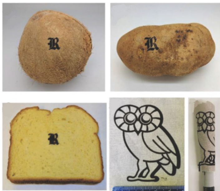
Figure 1.6: Different substrates that have been employed to produce LIG which enables a variety of applications. Reprinted from [43] with permission from ACS Nano.
