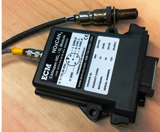
Figure 2.4: electrochemical fast NO x sensor and sensor control module
