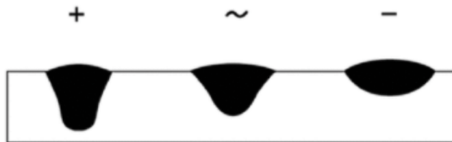
Figure 2.12 Effect of wire polarity on bead shape [37]
