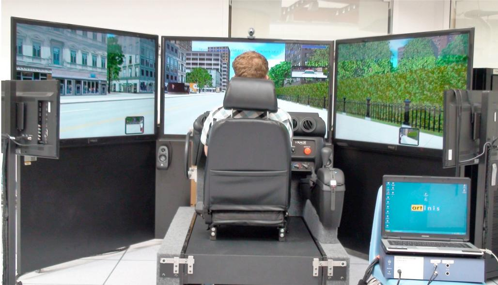
Equipment setup with VS500M (driving simulator) and Oxymon Mk III (NIRS collection device)
