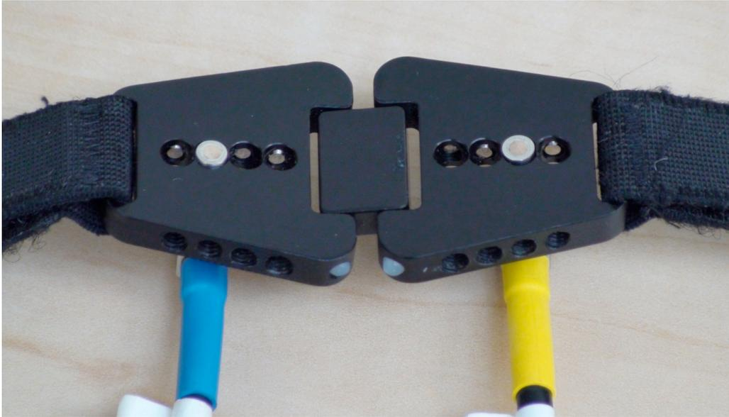
Close-up of NIRS optodes and optode holder. Transmitting optode is on the right and receiving optode is on the left. The inter-optode distance is 35 mm.
