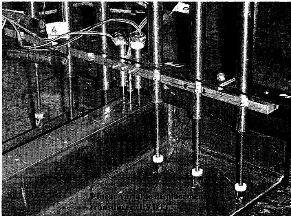
Figure 3.14 Layout of the Vertical Transducers for Initial Imperfections measurement
