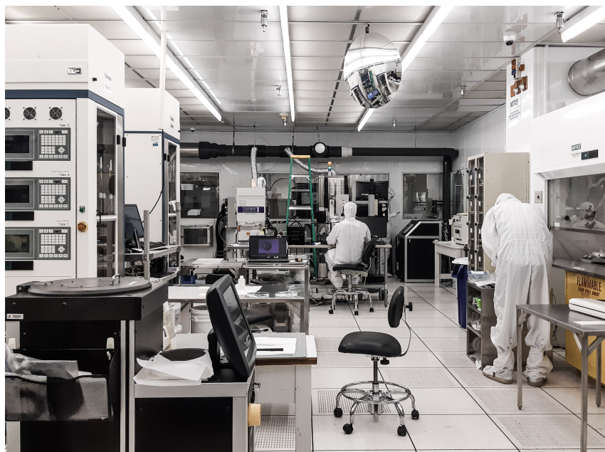
Figure 3.2 – Workers in the University of Alberta Nanofab’s class 100 cleanroom.
