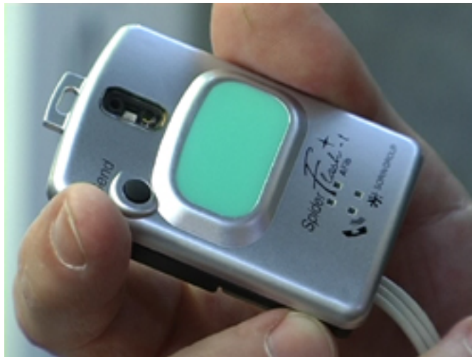
Figure 2. SpiderFlash-T ® (SFT ® ), the size is around 75×50×19 mm. (SORIN Group)
