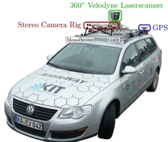
Figure 4.3: KITTI data acquisition setup [16].
