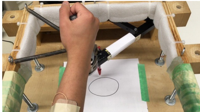
Figure 4-10 Figure showing the reproduction phase. The patient interacts with the robot to execute the given task, in the therapist's absence, the robot assists the patient to complete and perform the task just as the therapist did.
