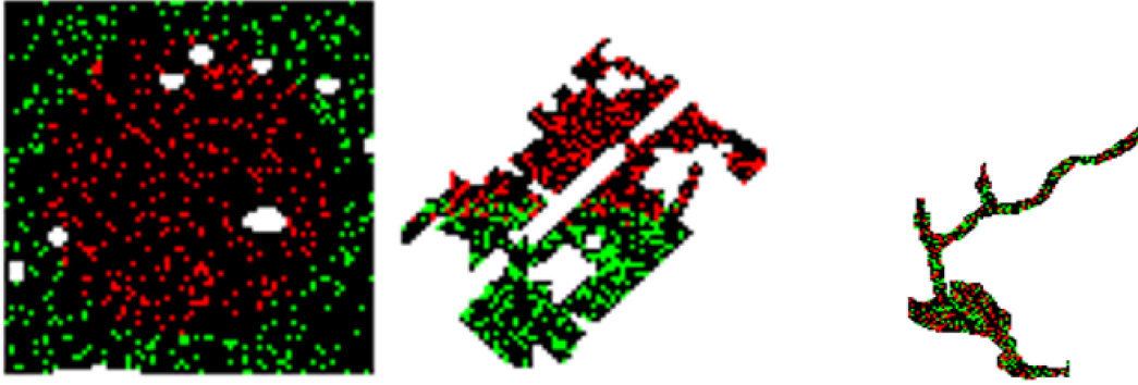
Figure 5.3: Three resized sample MAPF problem types with start (green pixels) and goals (red pixels): outside in (left), cross sides (centre), and switch sides (right).
