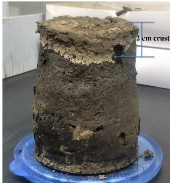
Figure 3.7: Crust layer formed at the surface of the centrifuged tailings subjected to a temperature gradient of  $0.028^{\circ}\text{C}/\text{mm}$
