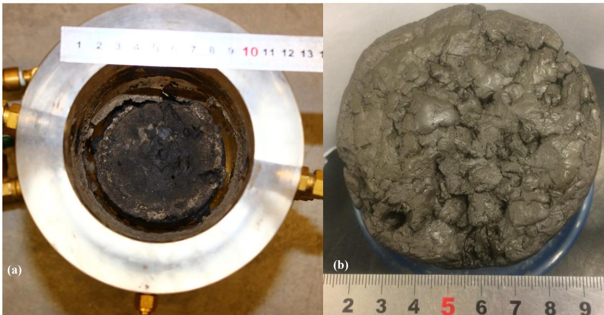
Figure 2.9: Photographs of drying-wetting test; 2.9a (left) shrinkage and cracking observed after drying test; and 2.9b (right) over-consolidated peds at the surface after wetting test
