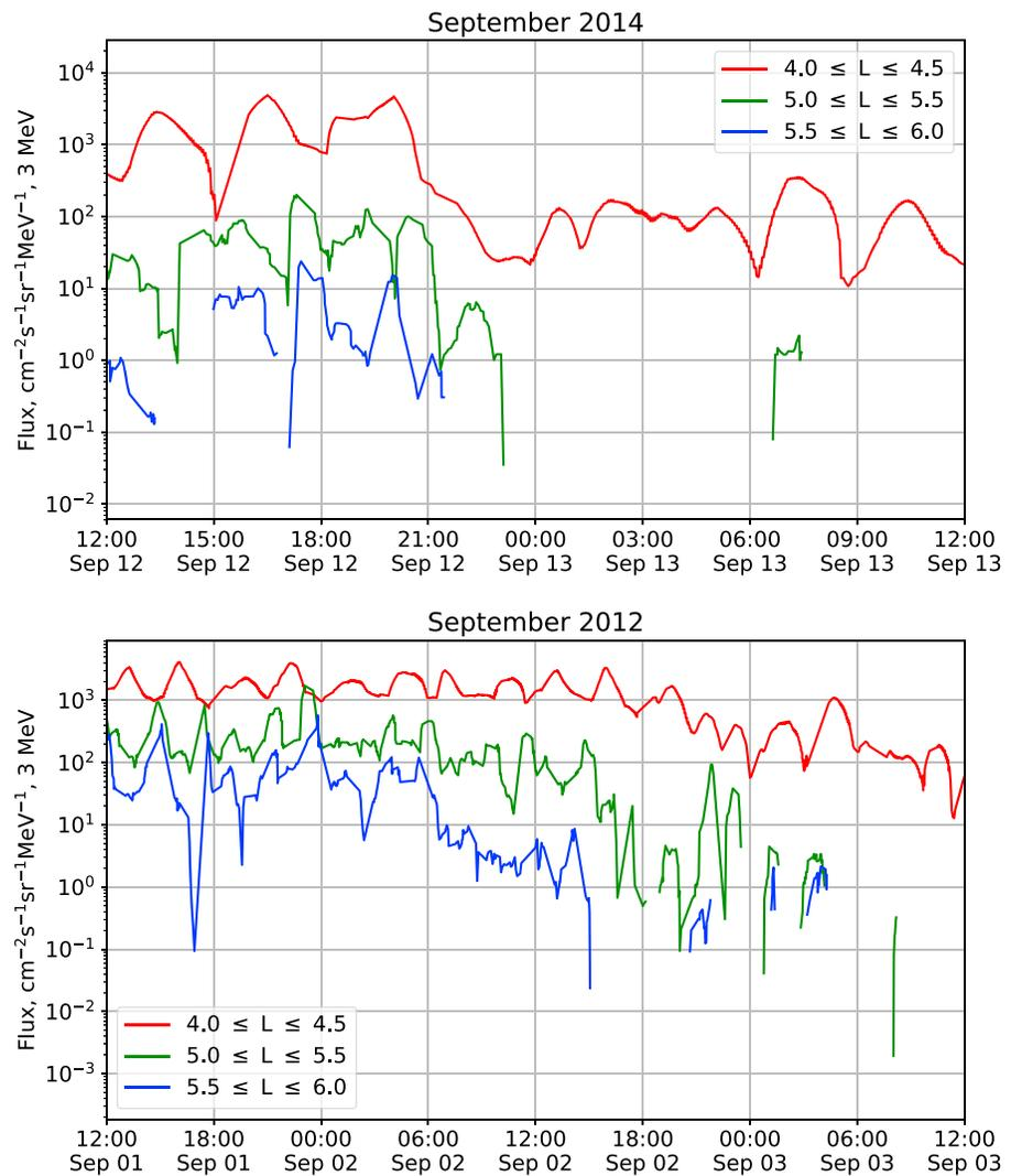
**Figure 7.** Time dependence of mean 3 MeV electron flux observed from the Global Positioning System satellite constellation binned in three L-shell ranges for the September 2014 and September 2012 storms. Note that only 24 hr of data is shown for September 2014, while 48 hr is shown for September 2012.
