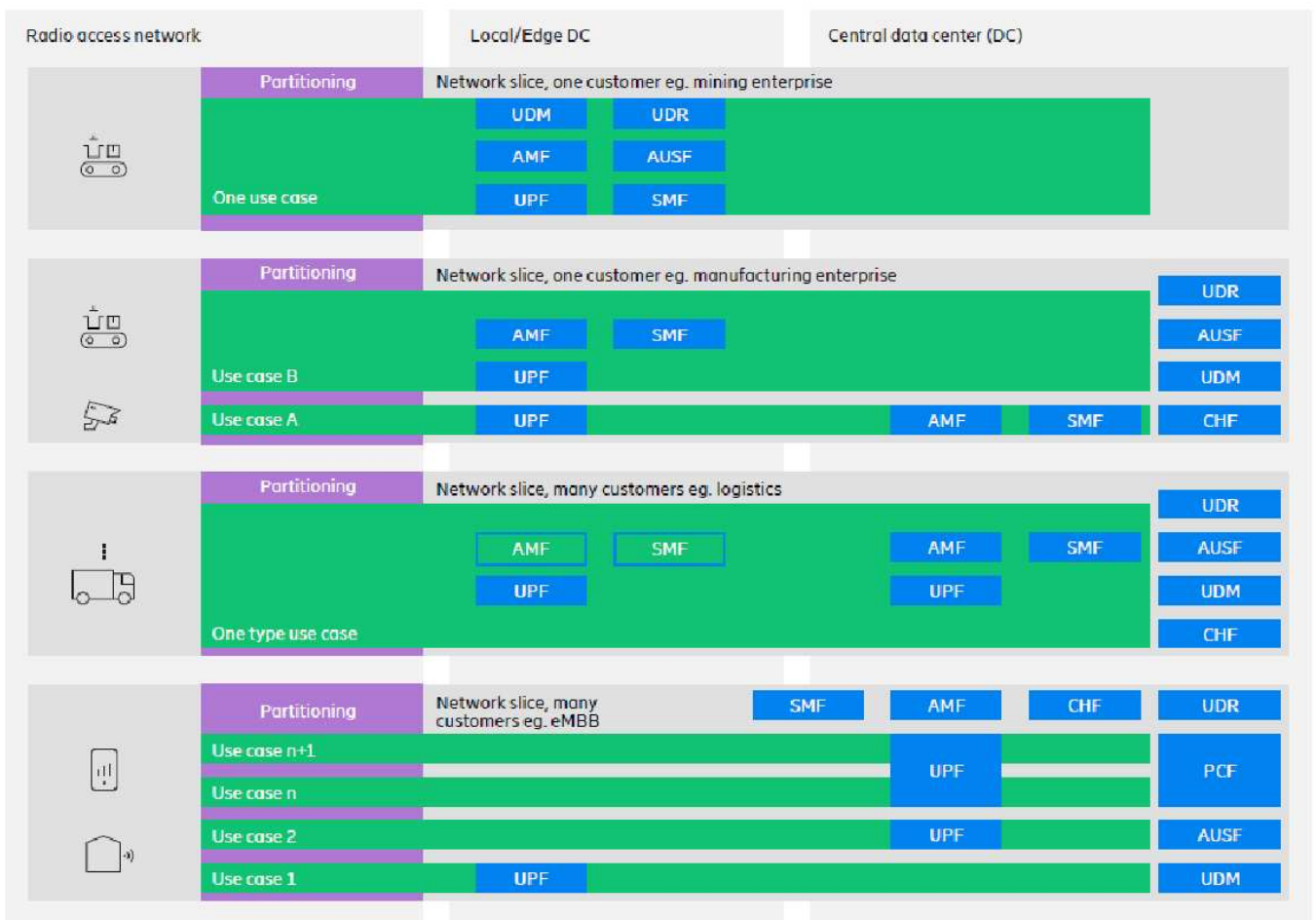
Figure 2-1. 5G network slicing catering for different and unique service needs [36]
