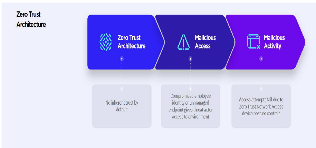
Figure 3-3. Attack Scenario on Zero Trust Architecture [53]
