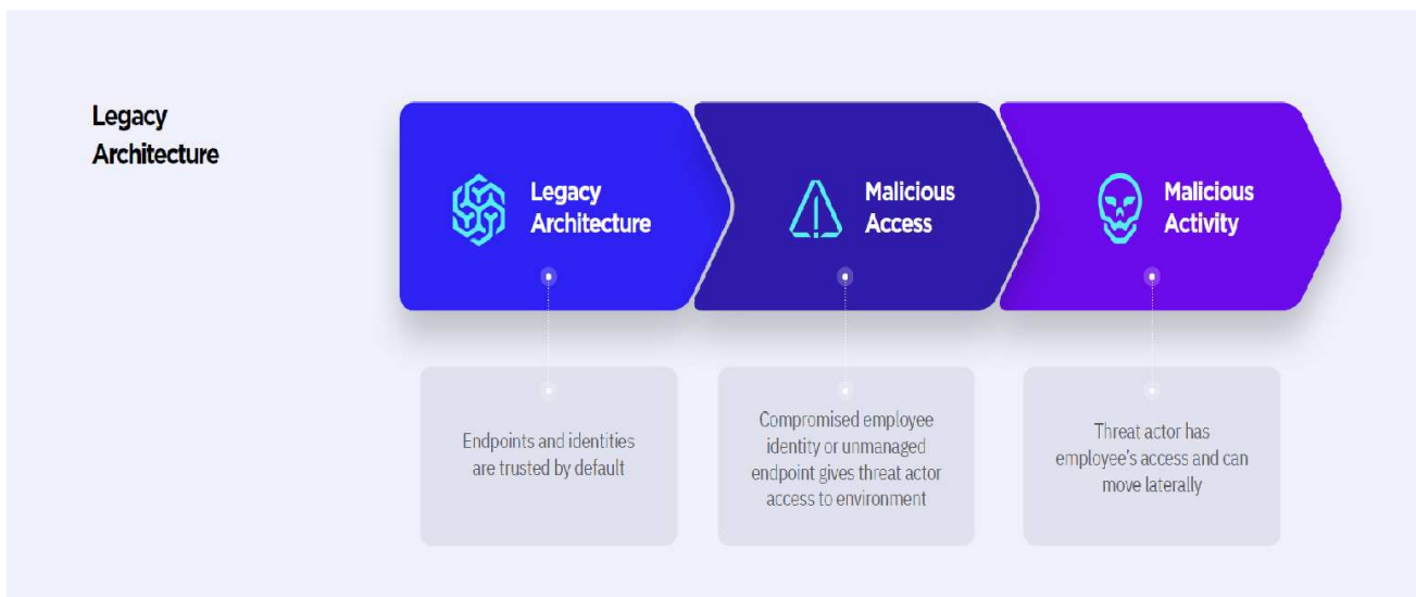
Figure 3-2. Attack scenario on legacy security architectures [53]
