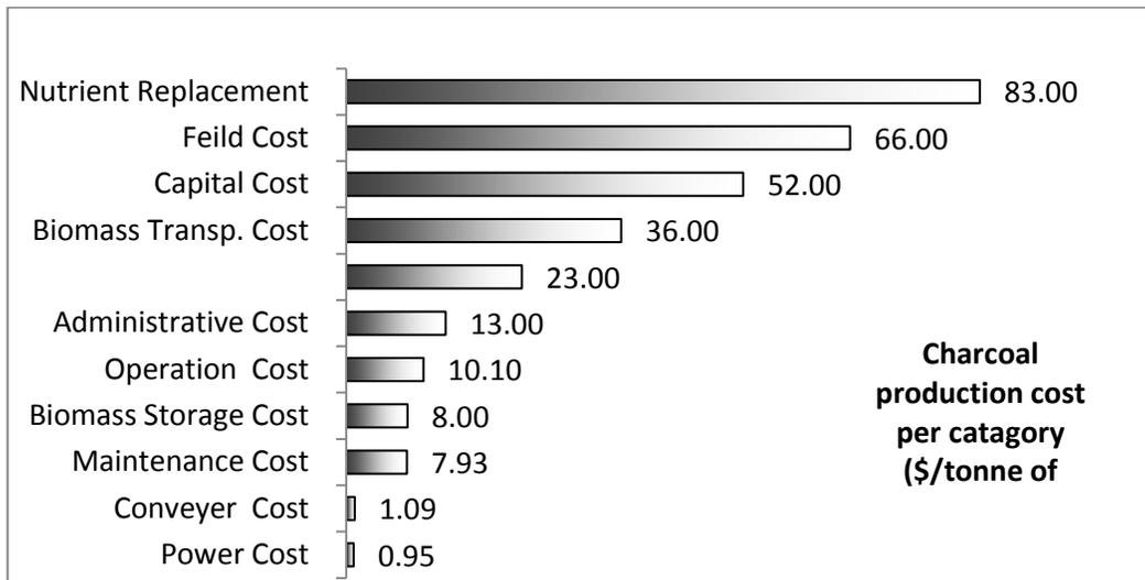
**Figure 2-4: Breakdown of charcoal production cost (\$/tonne of charcoal)**
