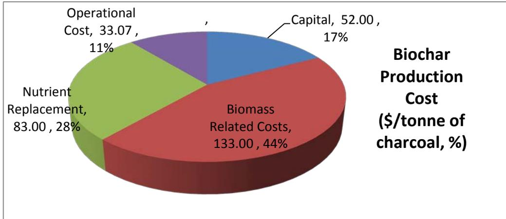
**Figure 2-3: Biochar production cost break-down**
