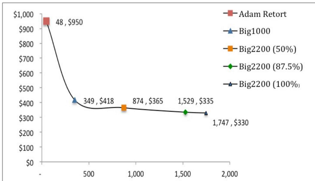
Figure 2-9: Various portable Biochar Equipment costs<sup>1</sup>
