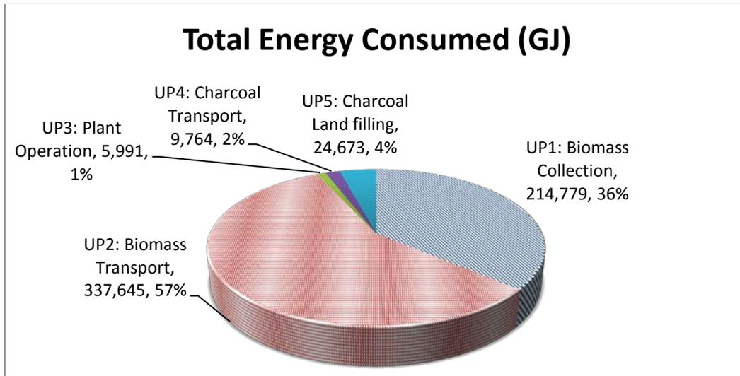
**Figure 3-4: Energy consumption in Charcoal production**
