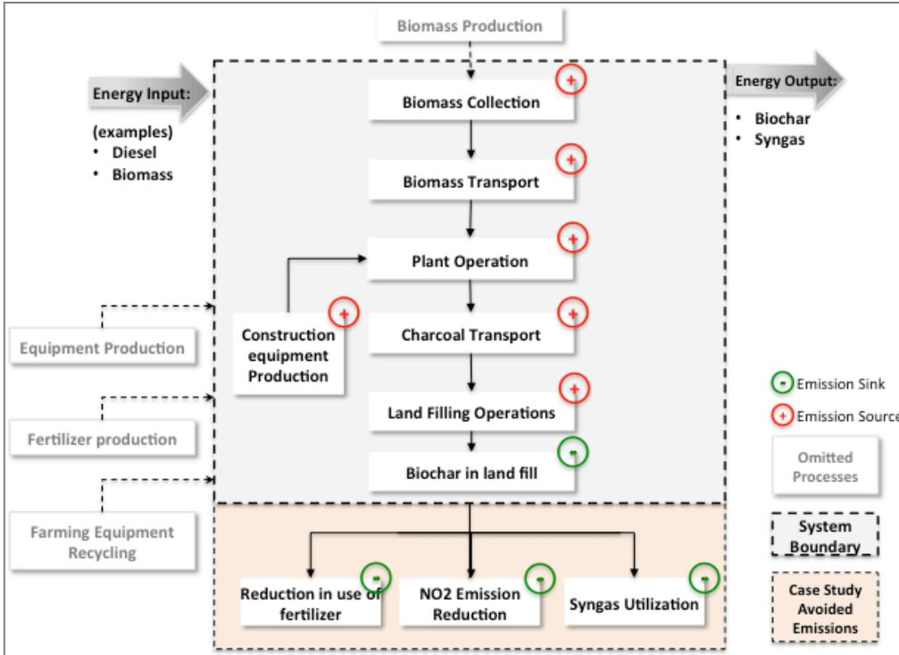
Figure 3-1: LCA and energy methodology
