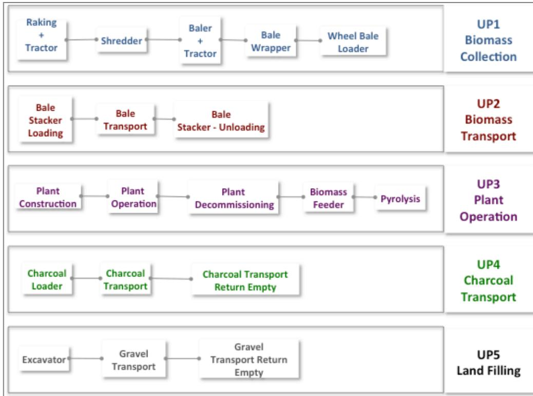
**Figure 3-2: Unit operations involved in charcoal production from agricultural biomass.**
