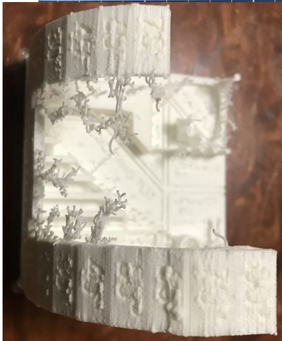
Figure 17. LW-PLA Test Structures. Top: Athena of Velletri. Bottom: Mini All-in-One Printer Test.
