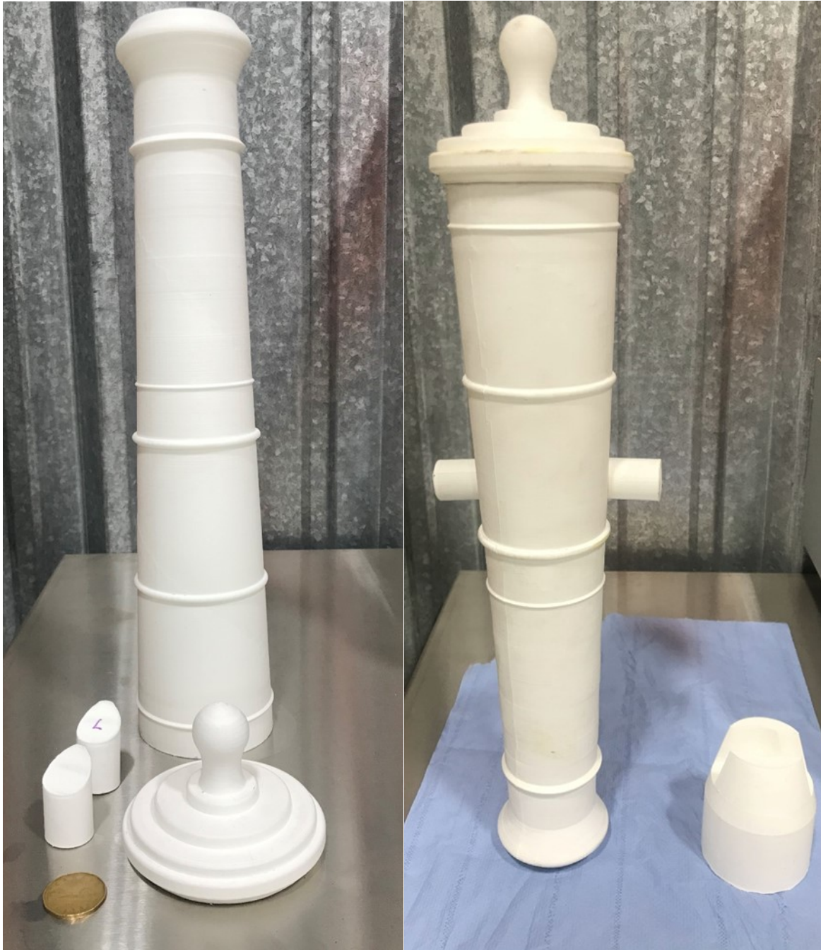
Figure 20. Expendable medieval cannon pattern. Left: before assembly. Right: partially assembled. The split sprue is shown at the bottom right.
