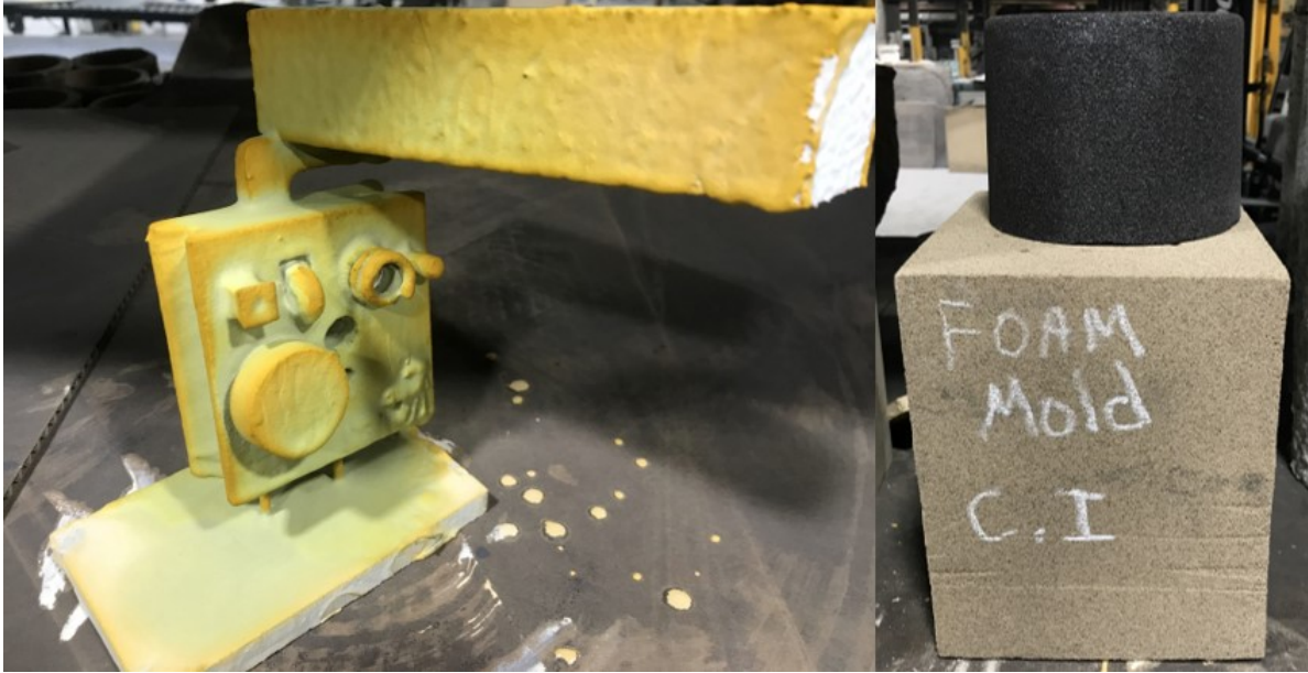
Figure 22. Left: Test pattern coated with Holcote 3100. Right: Test pattern molded in sand.
