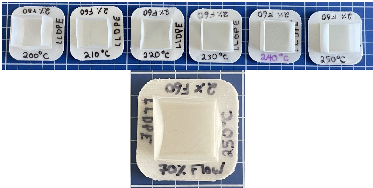
Figure 27. Top: LLDPE-F Test shells at 2 % F60 loading. Bottom: Optimized flow rate to achieve a wall thickness of 0.4 mm.
