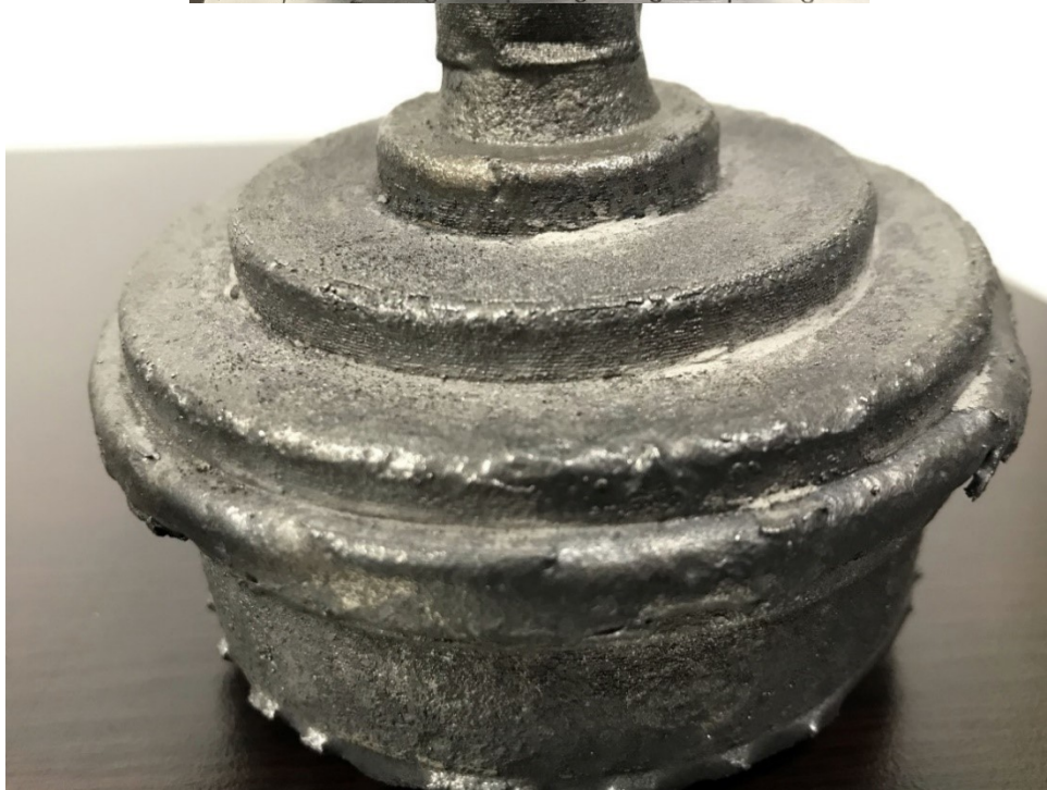
Figure 25. Medieval cannon casting. The level of detail replication is high, with layer lines visible.
