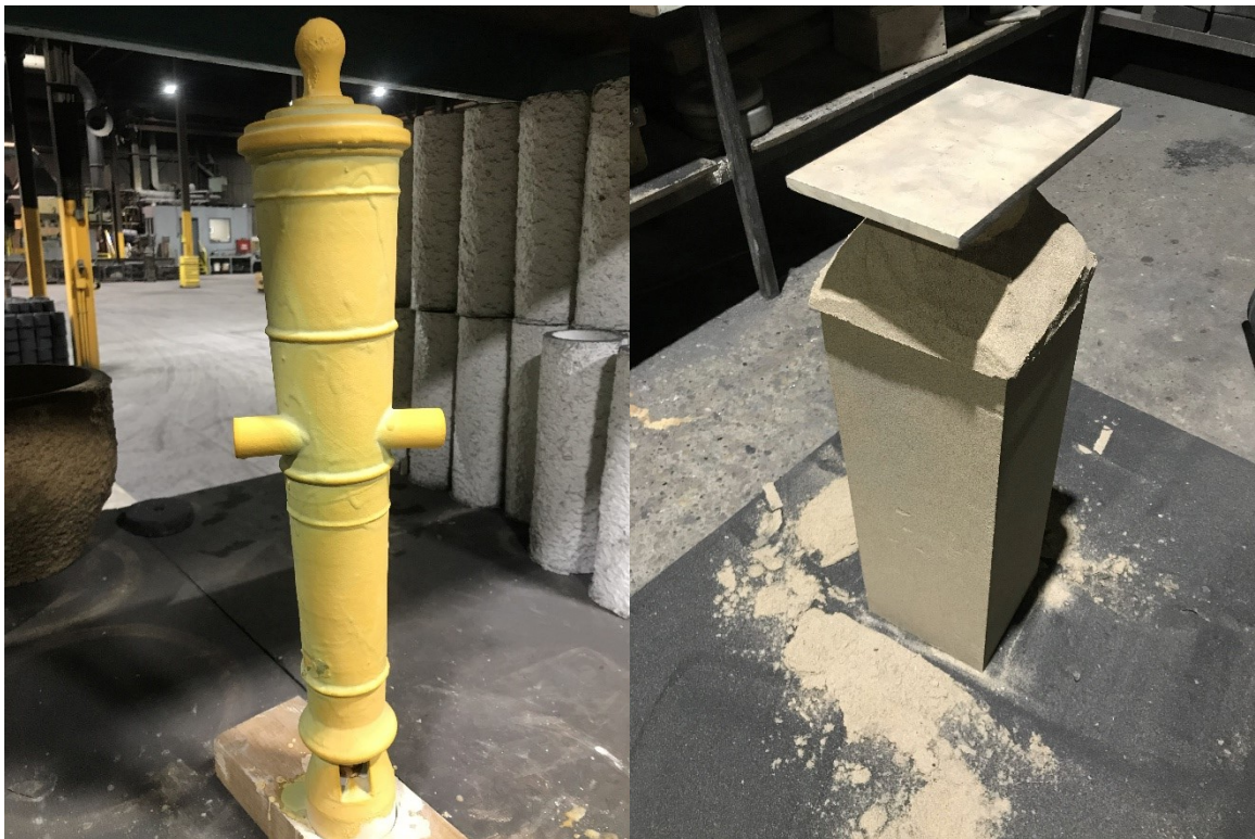
Figure 23. Left: Cannon pattern coated with Holcote 3100. Right: Cannon pattern molded in sand.
