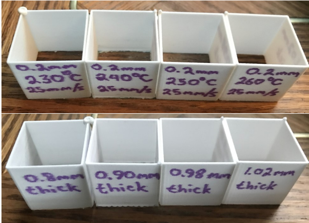
Figure 16. LW-PLA Calibration Shells.
