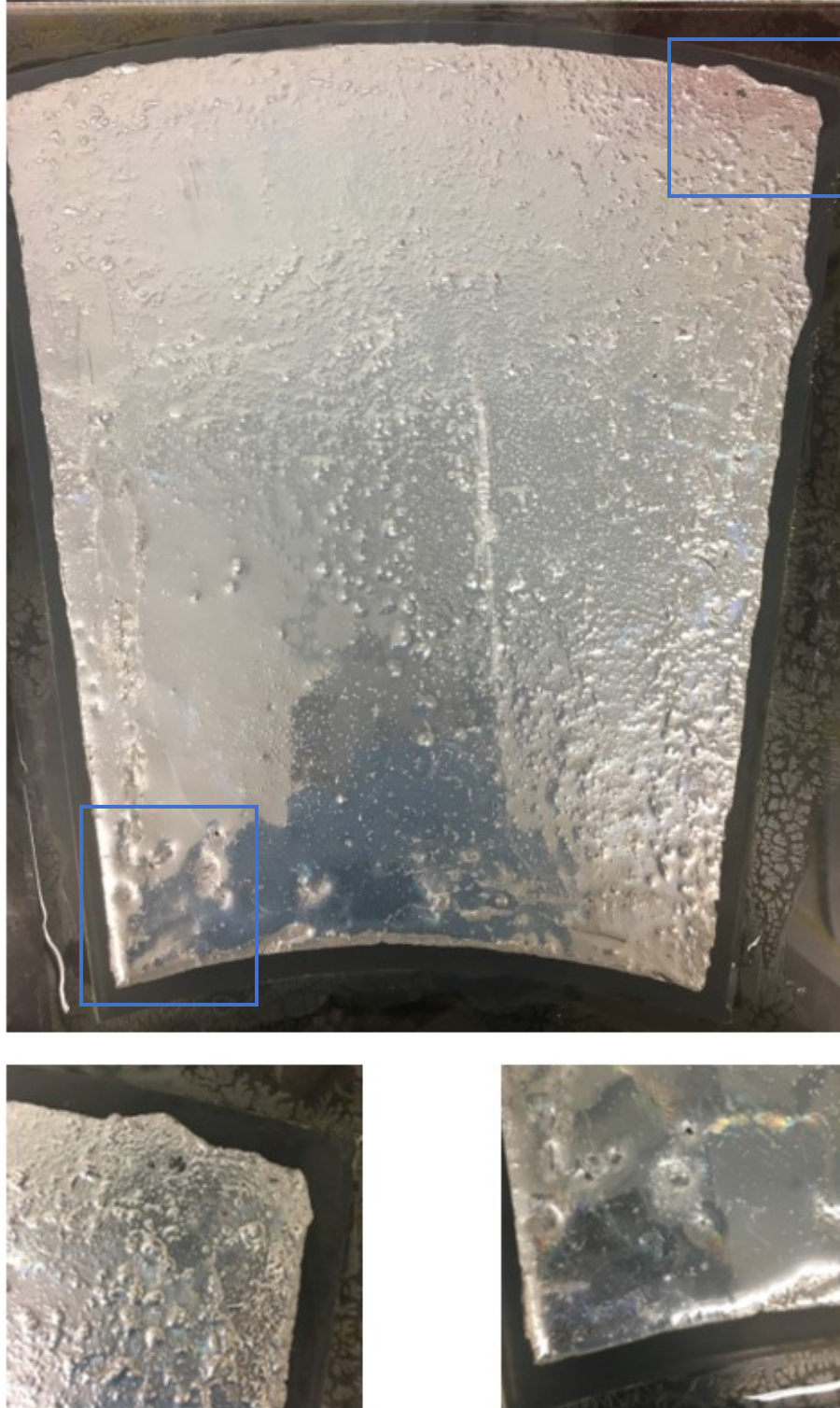
Figure 42. Reflector containing eGaIn prior to top layer lamination. Left inset: eGaIn that overflowed and penetrated between the paper mask and EcoFlex. Right inset: Oxidized eGaIn around air bubble pockets.
