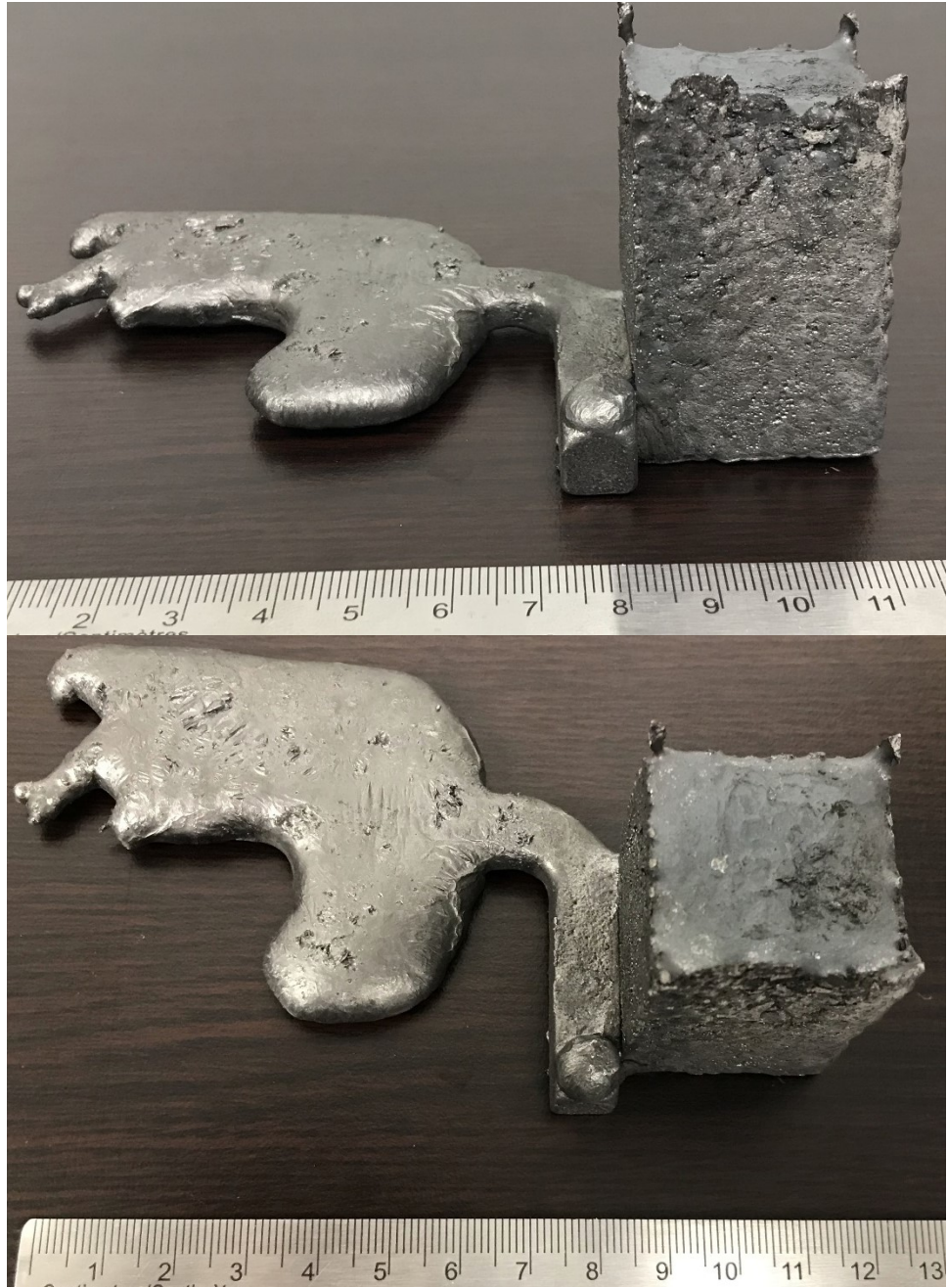
Figure 24. Test pattern casting. The EPS downsprue and the LW-PLA runner are visible.
