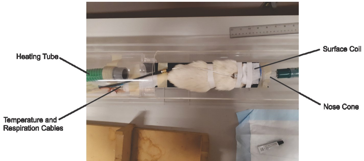
Figure 2.17: Rat brain spectroscopy setup with heating tube, nose cone, and temperature and respiration cables, along with the surface coil placed over the rat's head.
