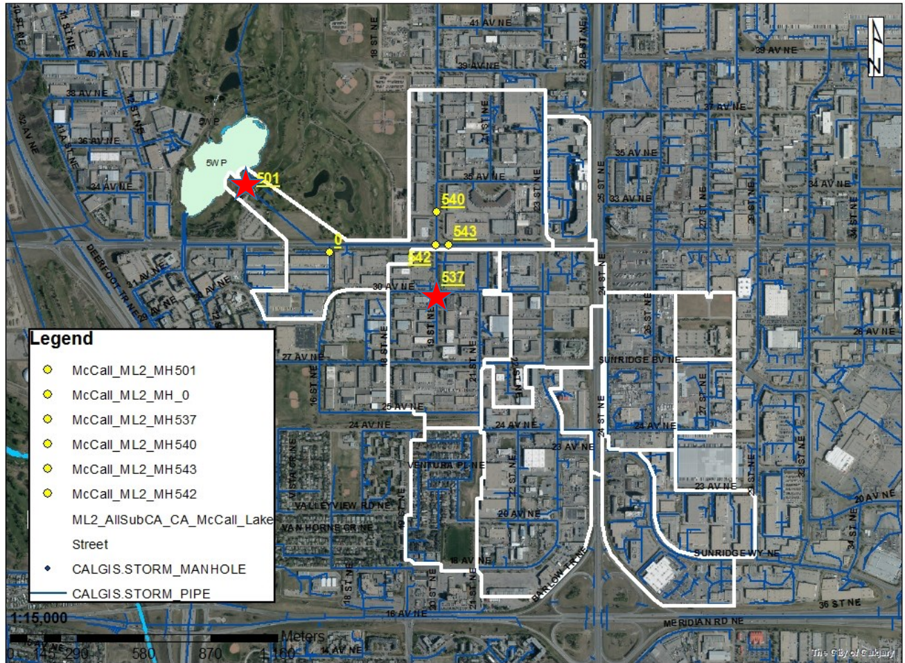
Figure 4-7: Map of the drainage network for ML2 from special investigations. The red stars indicate points where human fecal contamination was detected. Manhole 501 and manhole 537 were both tested in special investigation #1 and were positive.
