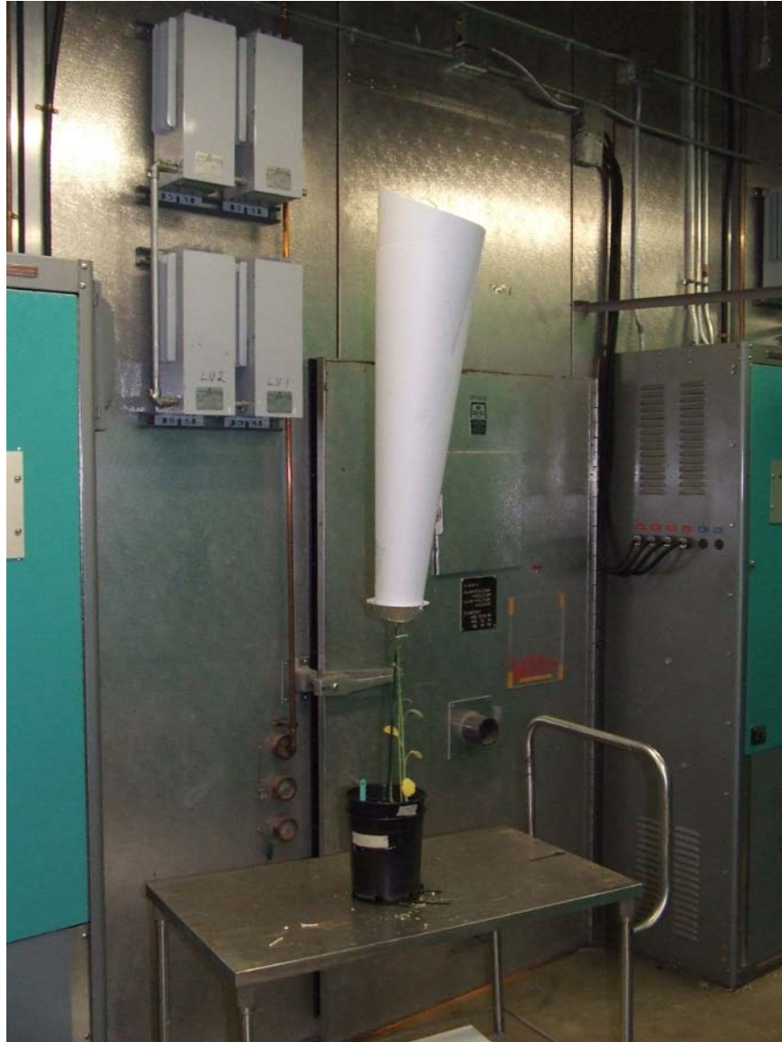
Figure 2.4. The cone and collecting plates used to capture emerging final instar larvae in the larval growth and development experiment.
