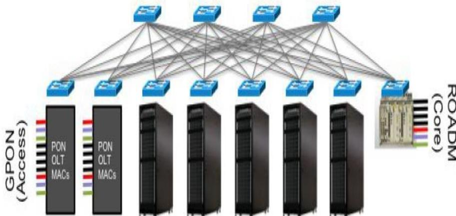
**Figure 1: Hardware Built From Commodity Server, I/O blades and switches**
