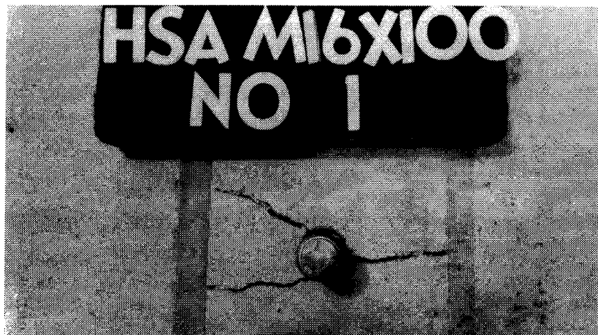
Plate 3.15 Tension Failure in Masonry
