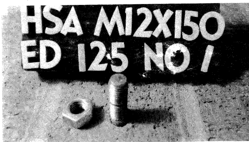
Plate 3.27 Tension Failure Under Embedment Depth Test
