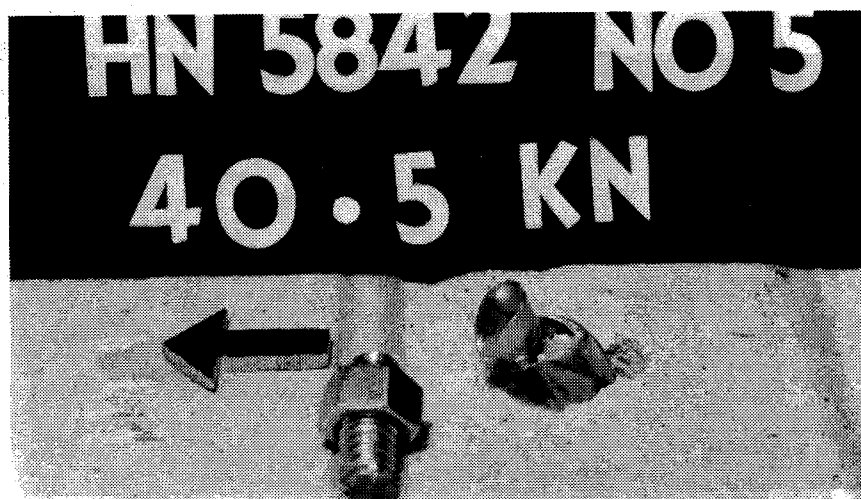
Plate 3.10 Insert Failure in Shear
