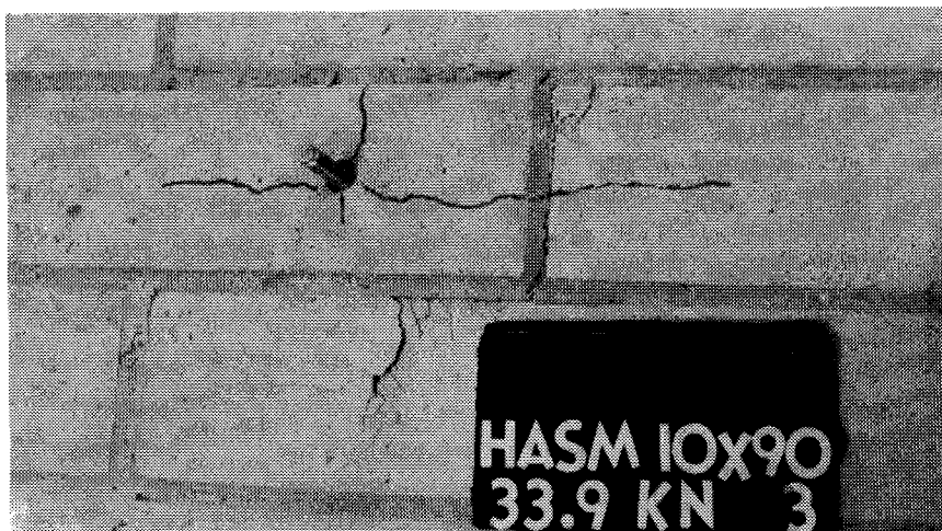
Plate 3.12 Tension Failure in Masonry
