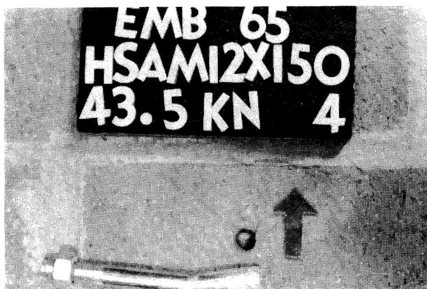
Plate 3.24 Shear Failure Under Embedment Depth Test
