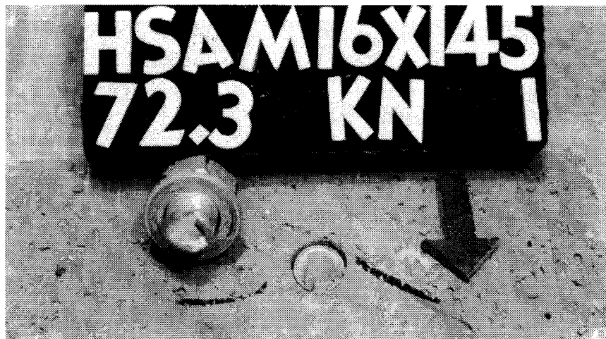
Plate 3.6 Insert Failure in Shear
