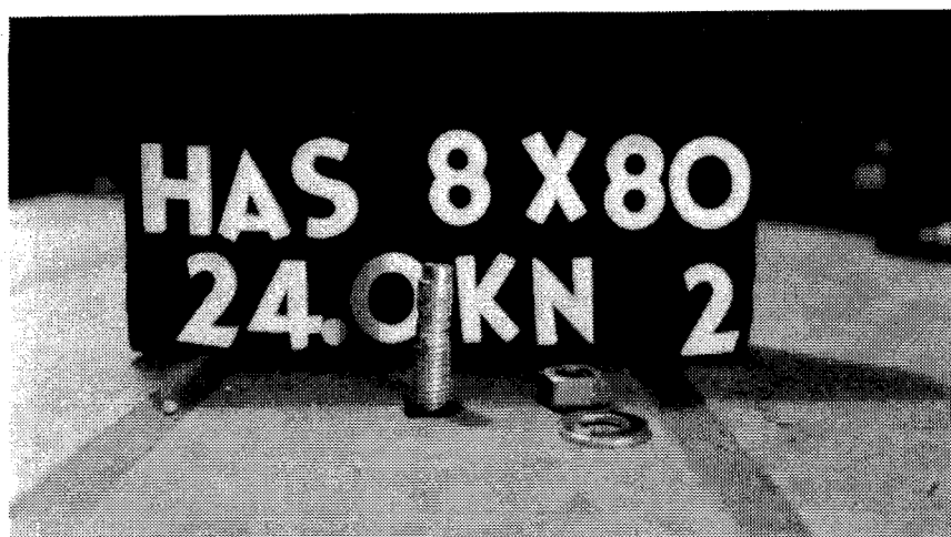
Plate 3.13 Threads Stripped in Tension Test
