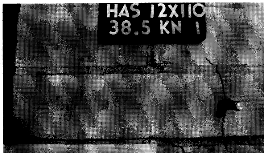
Plate 3.14 Tension Failure in Masonry (HAS = HVA)
