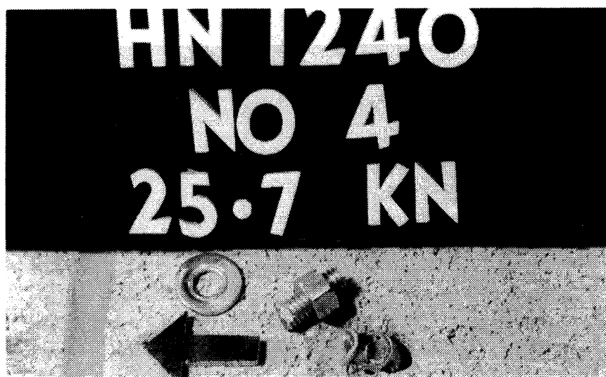
Plate 3.11 Insert Failure in Shear
