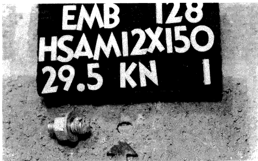
Plate 3.21 Shear Failure Under Embedment Depth Test
