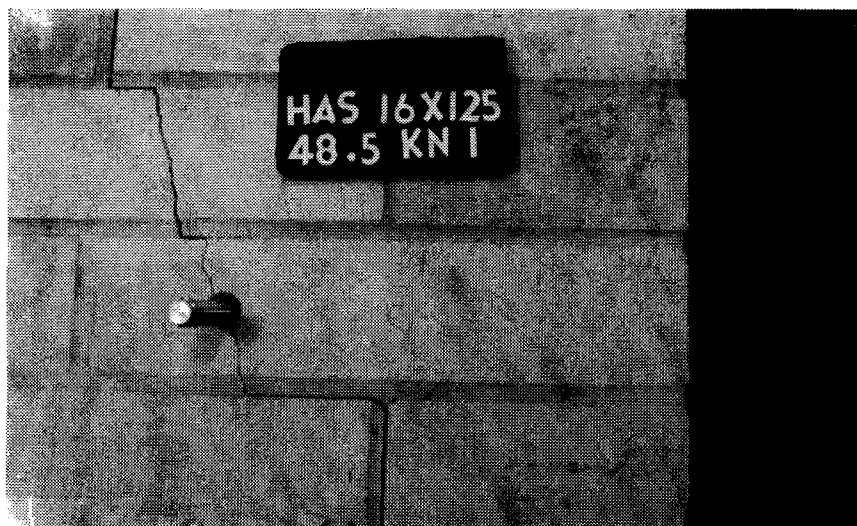
Plate 3.16 Tension Failure in Masonry (HAS = HVA)
