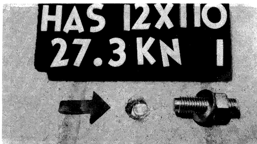
Plate 3.7 Insert Failure in Shear
