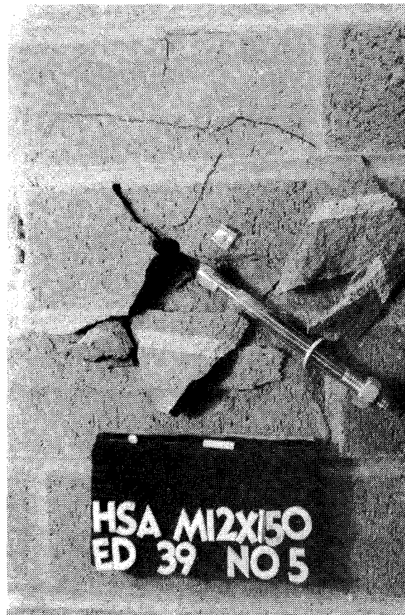
Plate 3.30 Tension Failure Under Embedment Depth Test
