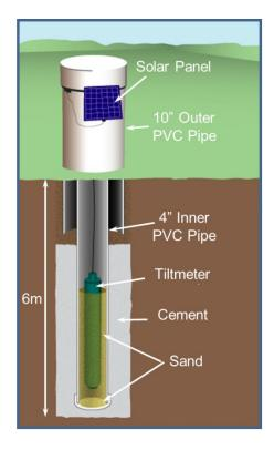
Figure 2-14 Scheme of tiltmeter installation
