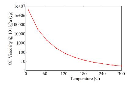
Figure 5-5 Bitumen viscosity vs. temperature relationship used in simulation
