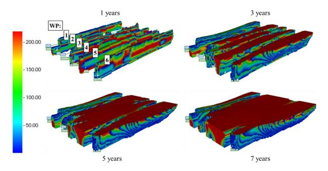
Figure 5-7 3D Steam chambers geometry from thermal reservoir simulation
