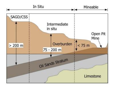
Figure 2-2 Schematic cross-section of Northeast Alberta sedimentary basin—originally published in (awrl.ca)
