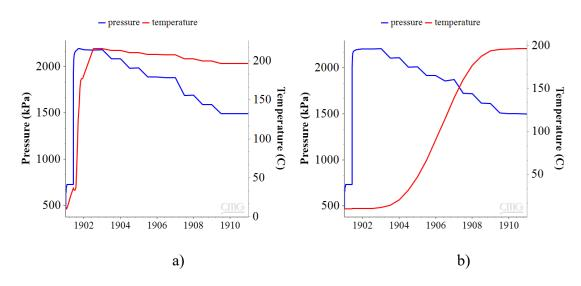
Figure 5-15 Pressure and temperature behavior at two different locations within the reservoir. a) a few meters away from a well-pair. b) At the middle of two well-pairs.
