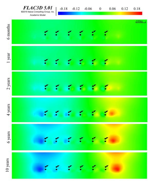
Figure 5-17 2D cross-section of horizontal displacement perpendicular to wells' trajectories for different times.
