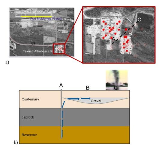
Figure 2-4 Blowout Texaco Fort McMurray Airport (a) aerial photographs of the patterns originally published in Livesey (2013) (b) Cross-section scheme of the project and flow pathway.
