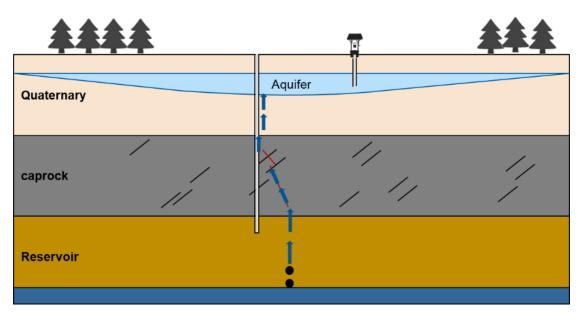
Figure 1-3 Different pathways that can be generated or opened during steam injection, allowing flow from the reservoir to the upper layers.
