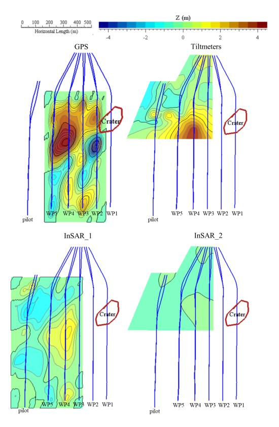
Figure 7-3 Vertical displacement measurements taken by different technologies 20 months after the project restart
