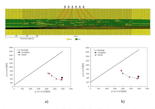
Figure 5-10 Stress path at two points in the middle of Pad in Clearwater formation. a) Silt in Clearwater b)Shale in Clearwater
