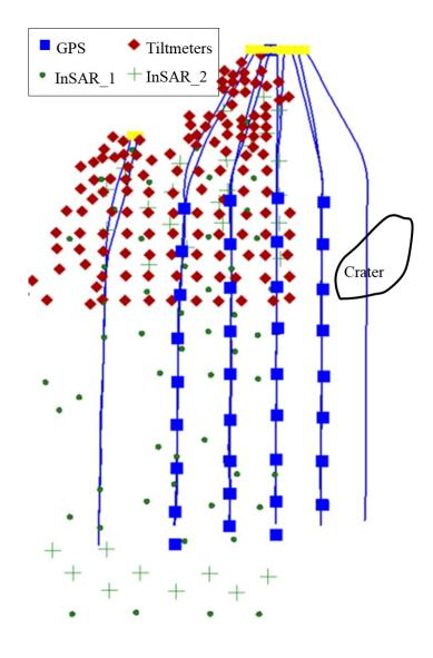
Figure 7-1 Heave monitoring instruments at Pad 204 Joslyn's SAGD Project after the 2006 blowout
