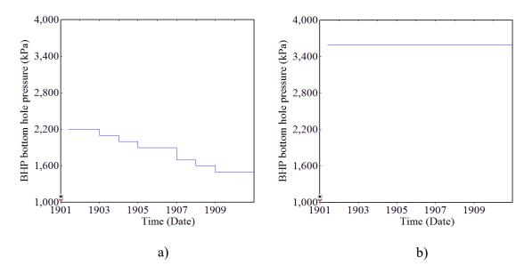
Figure 5-6 Injection pressure during SAGD. a) pressure below MOP. b) Pressure equal to minimum in-situ stress
