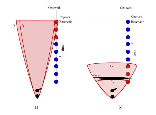
Figure 5-13 Temperature readings behavior at observation wells for a) homogeneous reservoir. b) heterogeneous reservoir
