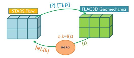
Figure 5-3 Sequential coupling simulation scheme (Deisman, 2017)
