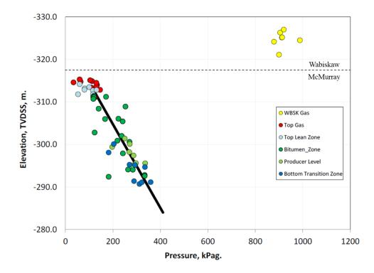
Figure 4-12 Initial pressure measurements at McMurray and Wabiskaw Formations. Modified from (Petrochina Canada, 2018)
