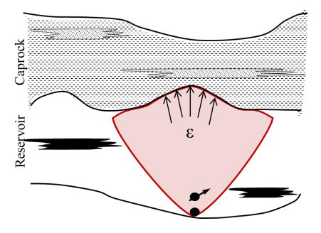
Figure 6-2 Schematic of conditions to initiate fracture in the caprock
