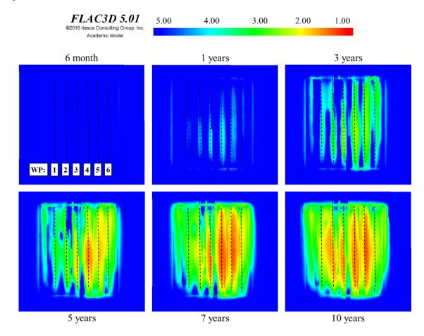
Figure 5-26 Safety factor at the base of caprock for SAGD below MOP
