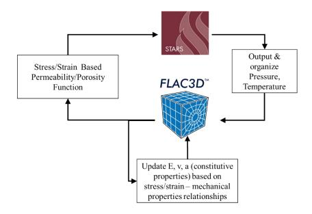
Figure 5-1 Reservoir Geomechanics Research Group coupling platform. Taken from Deisman (2017)
