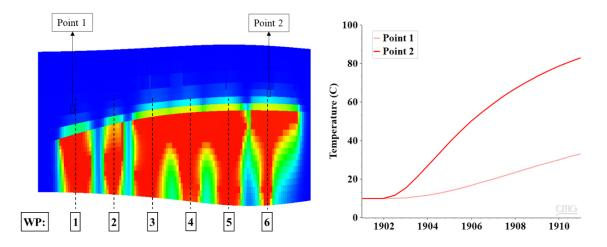
Figure 5-14 temperature behavior at the Wabiskaw sand monitoring zone.
