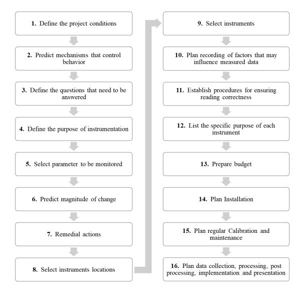
Figure 3-1 Workflow for systematic approach to designing geotechnical monitoring as proposed by Dunnicliff (Modified from Dunnicliff, 1988)
