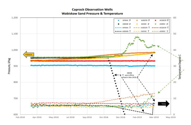
Figure 2-9 Temperature and pressure behaviour over time at Wabiskaw sand formation in PetroChina Canada's MacKay River project—originally pubplished in PetroChina Canada (2019)
