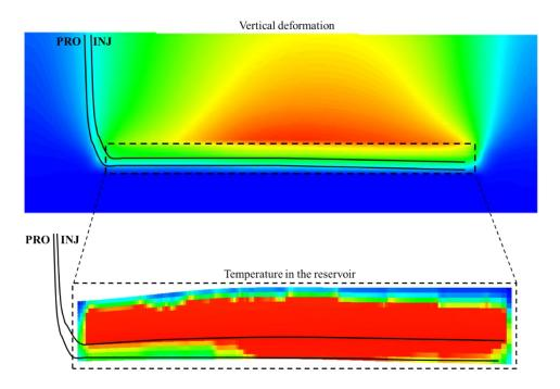
Figure 5-24 2D cross-section along Well-pair 6 for vertical displacement and temperature distribution within the reservoir.
