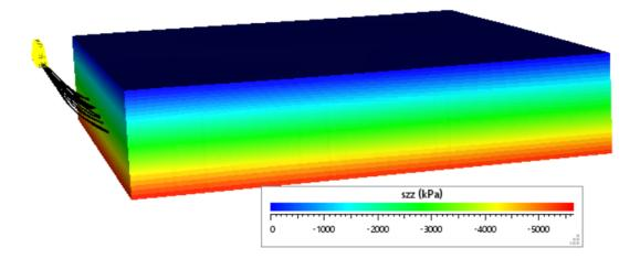
Figure 4-13 Calculated vertical stress at Pad AE model.
