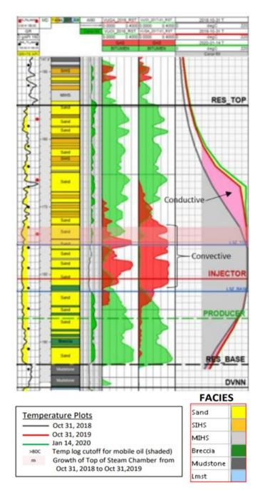
Figure 2-8 Typical temperature and saturations profile for Athabasca oil sands at three different times for Hangingstone Project, obtained from AER D54 2020 11888
