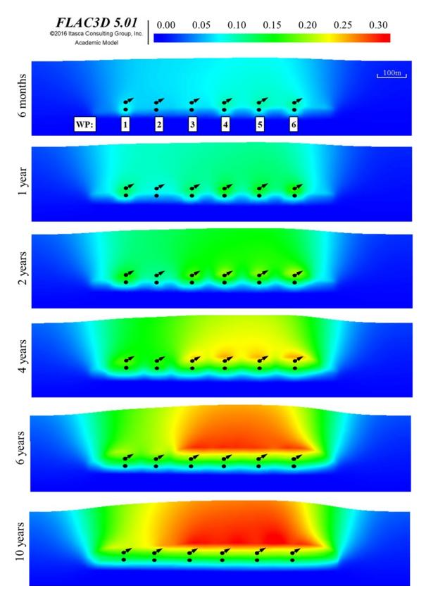
Figure 5-23 2D cross-section of simulated vertical displacement perpendicular to the well-pairs
