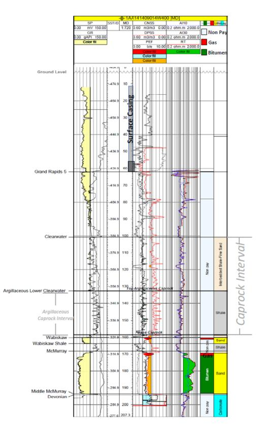
Figure 4-3 Typical stratigraphy and well logs in MacKay River Commercial Project area.
