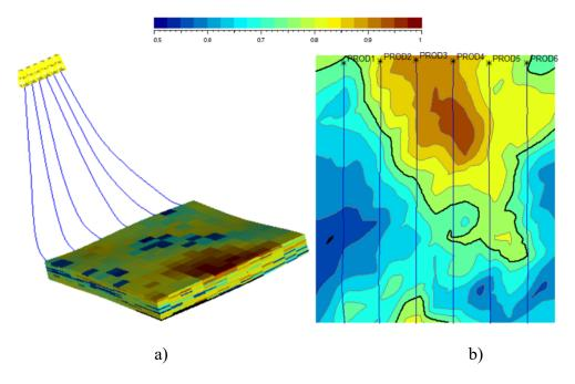
Figure 6-6 Reservoir Quality Index (CQI) for PAD AE at MRCP. a) 3D model of caprock with RQI for each cell. b) Aerial RQI map
