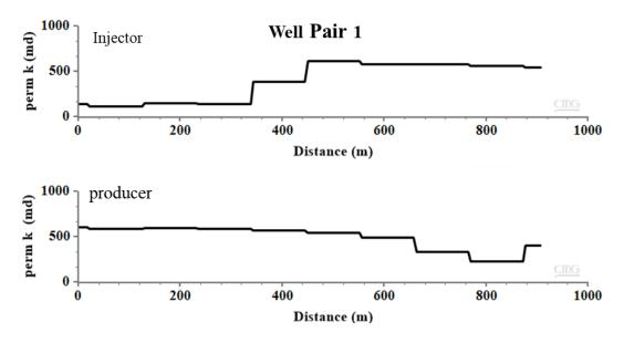
Figure 5-8 vertical permeability of blocks intersected by Well-pair 1.
