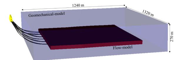
Figure 4-7 Flow model and Geomechanical model for Pad AE in MRCP.
