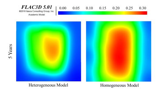
Figure 5-25 Simulated vertical displacements at the ground surface for homogeneous and heterogeneous models.
