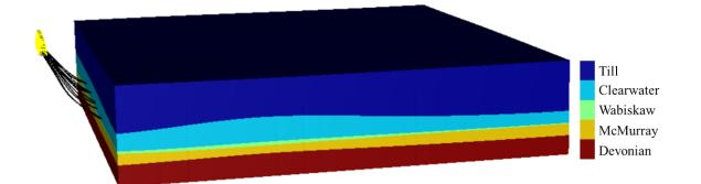
Figure 4-5 Layers constructed from horizons in the geomodel
