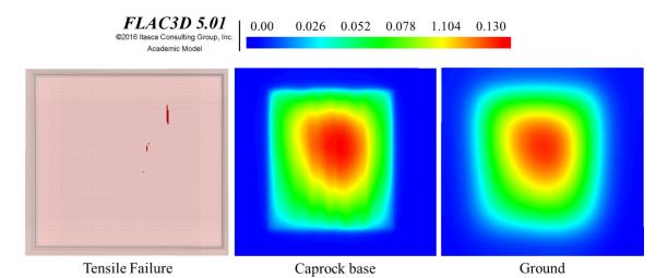
Figure 5-27 Tensile failure at the base of the caprock and vertical displacement at caprock base
