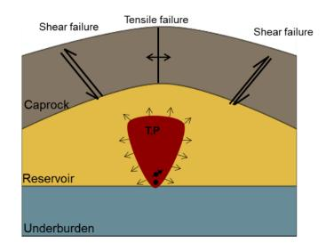
Figure 1-2 Schematic of possible failure mechanisms in the caprock during SAGD
