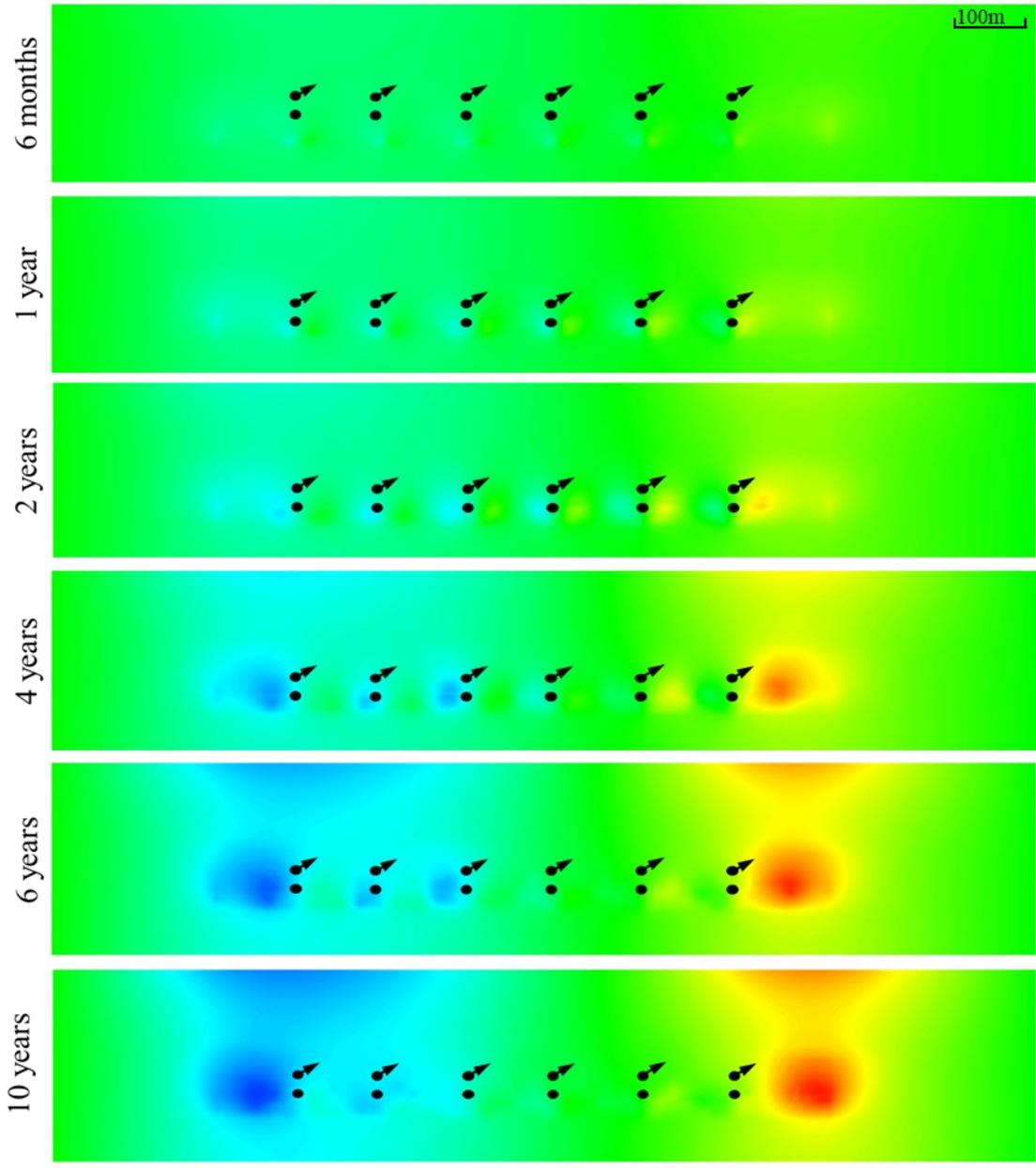
Figure 5-17 2D cross-section of horizontal displacement perpendicular to wells' trajectories for different times.
