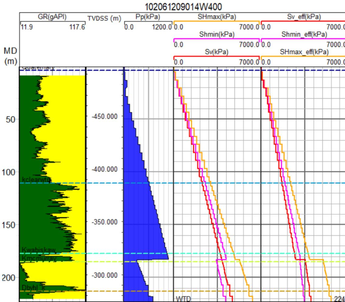
Figure 4-14 Pore pressure, total stress and effective stress profiles used in the model.
