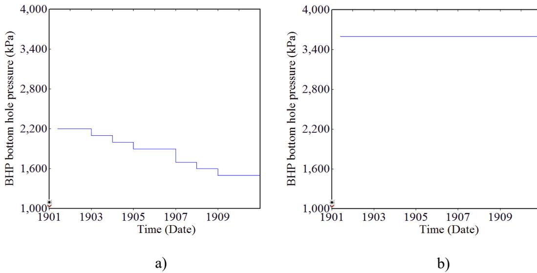
Figure 5-6 Injection pressure during SAGD. a) pressure below MOP. b) Pressure equal to minimum in-situ stress
