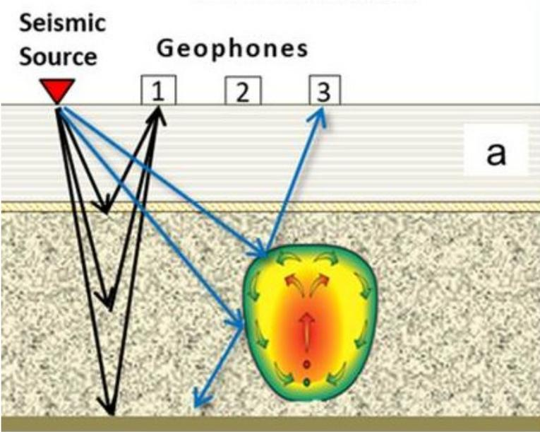
Figure 2-16 Schematic 4D seismic application during SAGD—obtained from (<https://www.nrcan.gc.ca/>)
