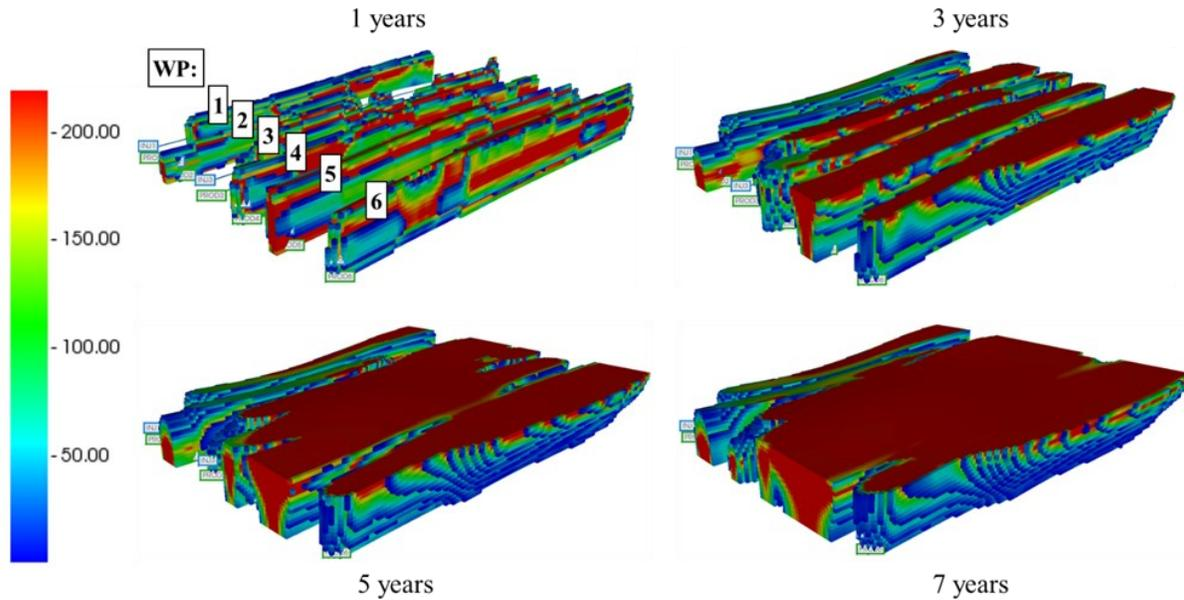
Figure 5-7 3D Steam chambers geometry from thermal reservoir simulation
