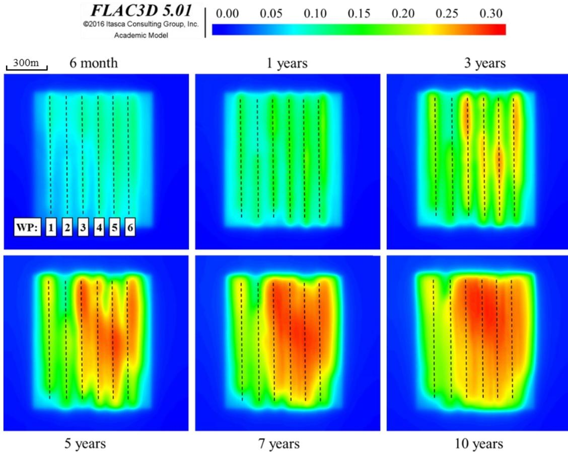
Figure 5-21 Simulated vertical displacement in meters at the base of the caprock during SAGD below MOP
