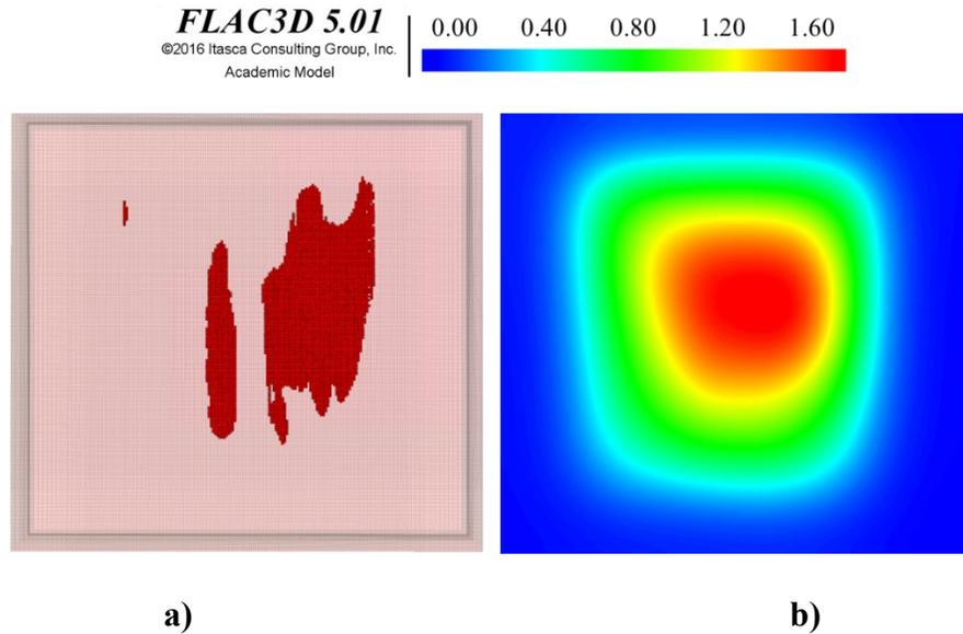
Figure 5-28 a) tensile failure after ten years of operation above MOP. b) Vertical displacement at the ground surface after ten years.
