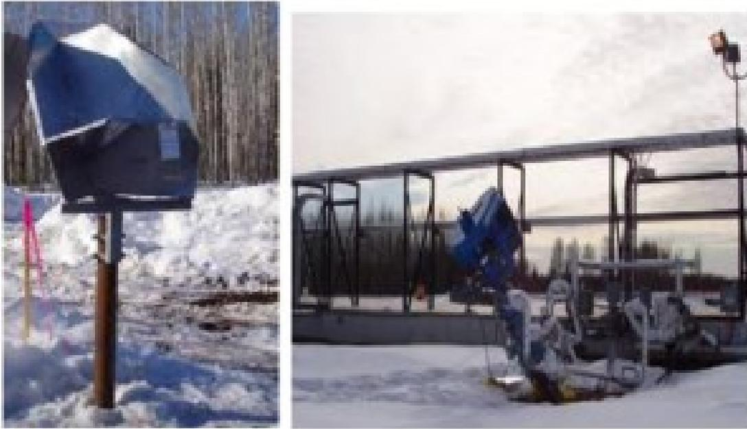
Figure 2-13 Corner reflector and natural reflectors from an oil field in Alberta—originally published in Tang et al. (2015)
