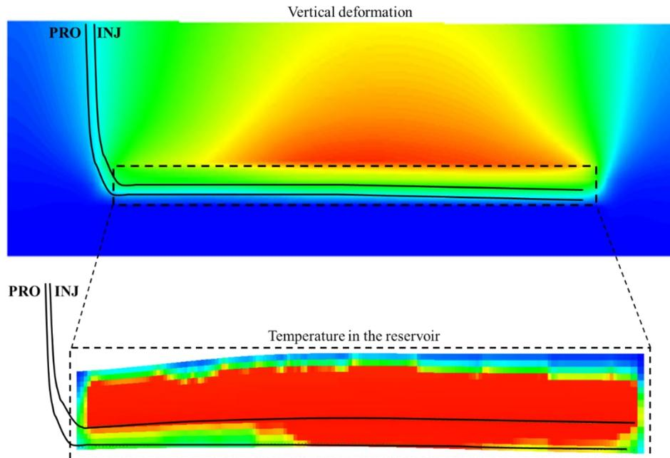
Figure 5-24 2D cross-section along Well-pair 6 for vertical displacement and temperature distribution within the reservoir.
