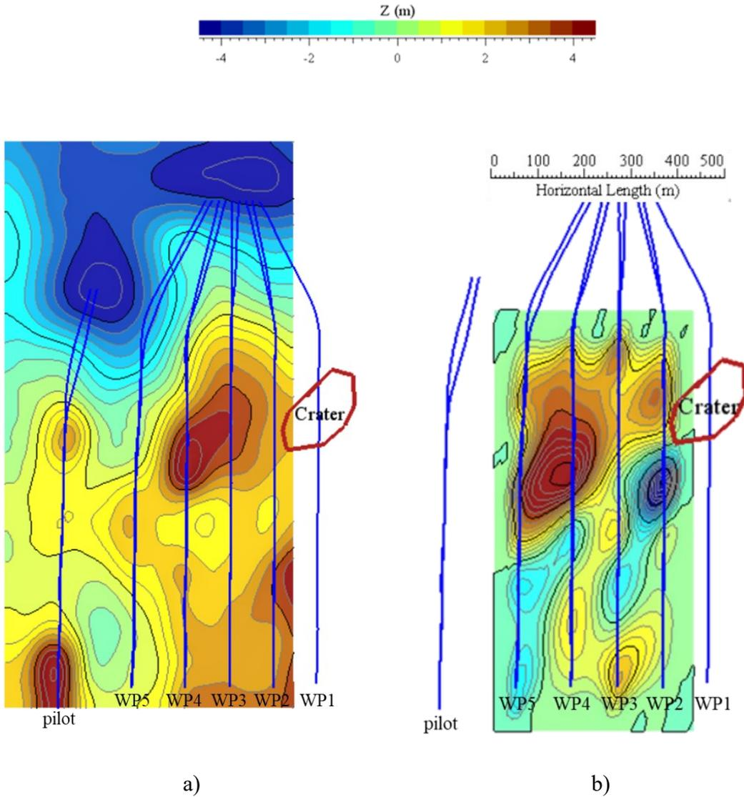
Figure 7-9 Surface heave, a) from numerical simulation, b) from D -GPS
