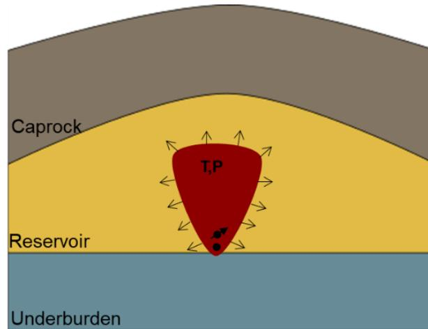
Figure 1-1 Steam chamber and deformation in the reservoir and surrounding formations
