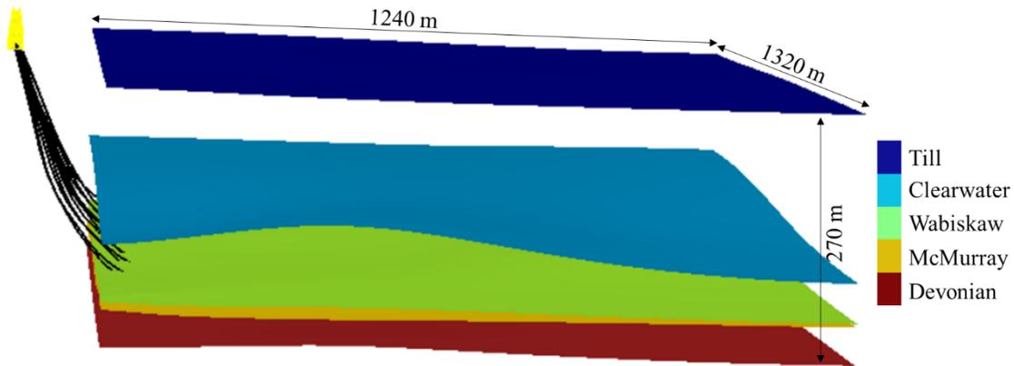
Figure 4-4 Stratigraphic horizons for Till, Clearwater, Wabiskaw, McMurray, and Devonian formations at Pad AE MRCP.
