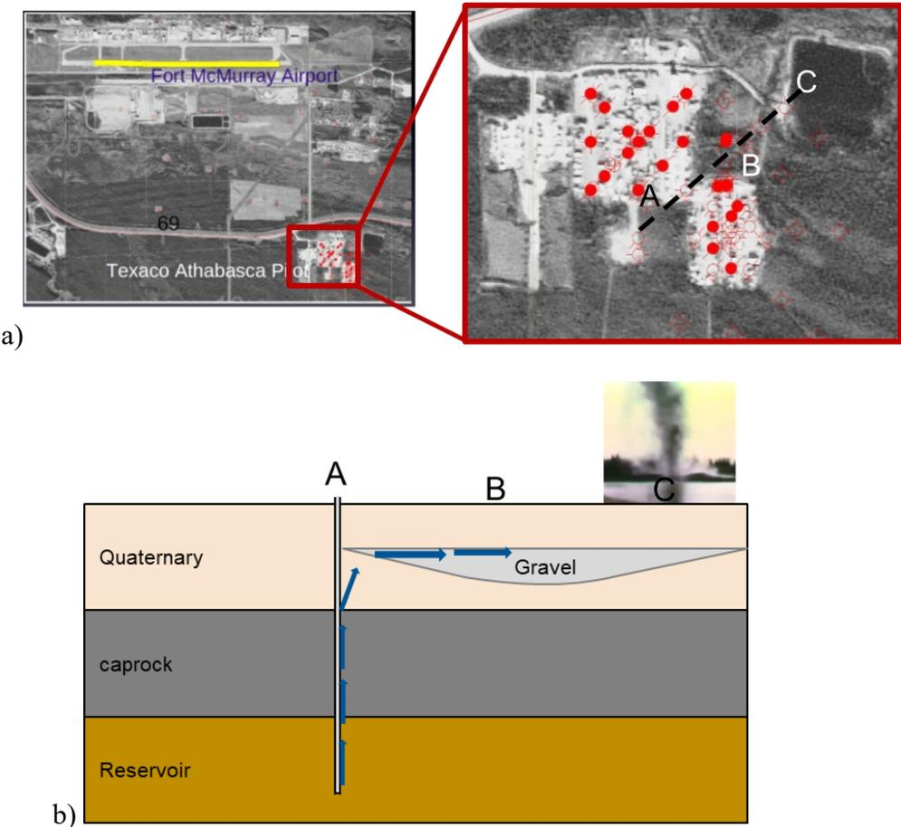
Figure 2-4 Blowout Texaco Fort McMurray Airport (a) aerial photographs of the patterns—originally published in Livesey (2013) (b) Cross-section scheme of the project and flow pathway.
