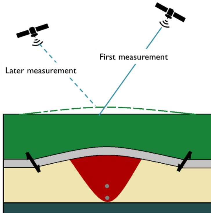
Figure 2-12 Schematic showing INSAR monitoring in SAGD.
