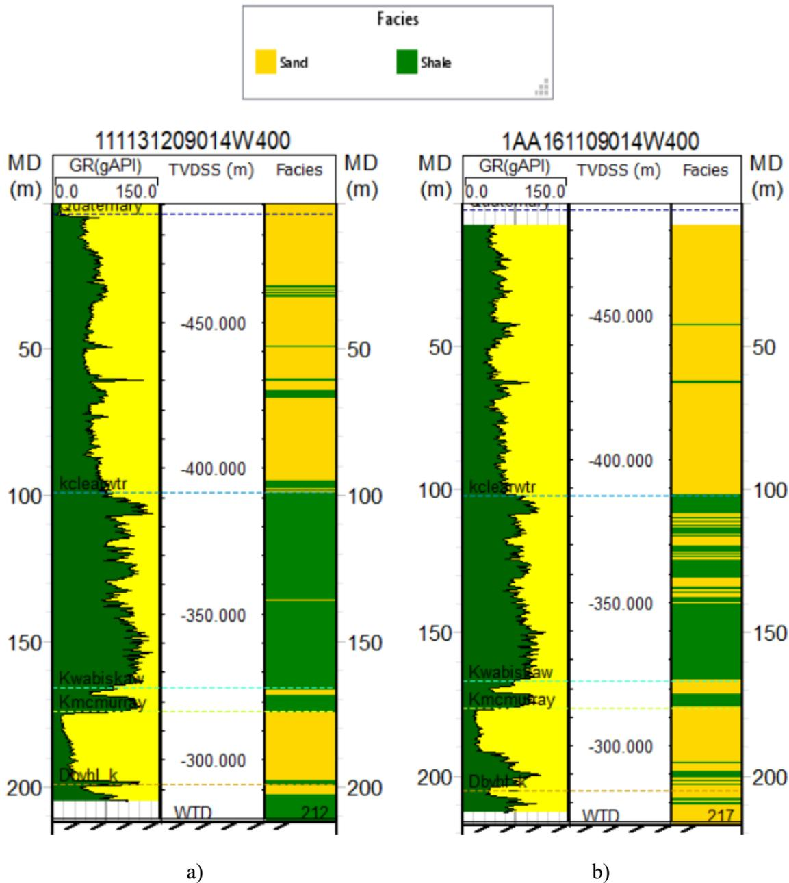
Figure 4-10 Gamma Ray and Facies distribution for two different wells.
