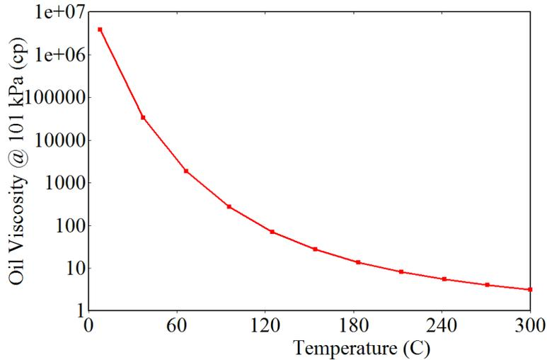
Figure 5-5 Bitumen viscosity vs. temperature relationship used in simulation
