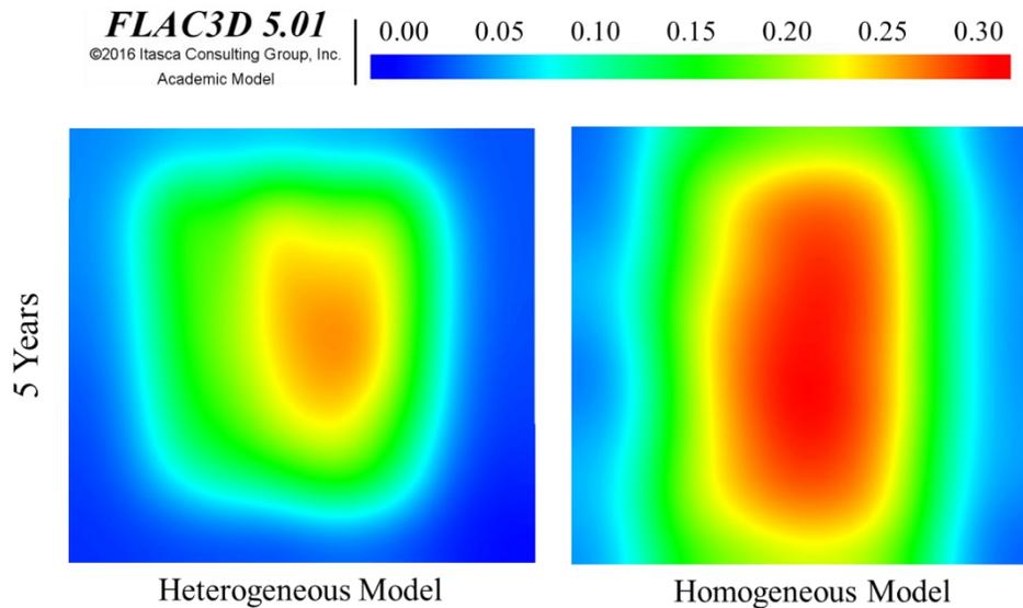
Figure 5-25 Simulated vertical displacements at the ground surface for homogeneous and heterogeneous models.
