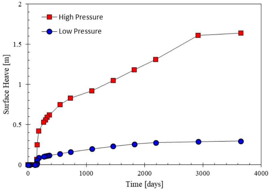
Figure 5-29 Comparison of predicted surface heave for SAGD operating below MOP and above MOP.
