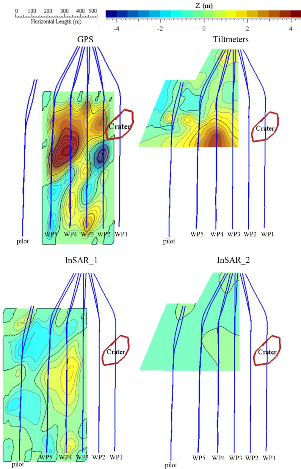
Figure 7-3 Vertical displacement measurements taken by different technologies 20 months after the project restart
