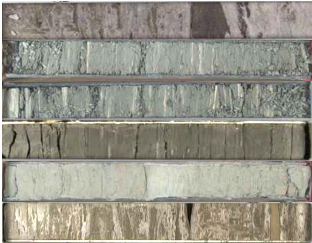
Figure 6-3 Photos of Clearwater Formation cores from Joslyn's thermal project. Taken from (Energy Resources Conservation Board, 2010)
