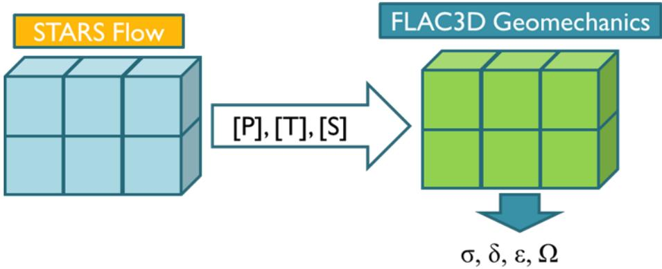
Figure 5-2 One-way coupling simulation scheme (Deisman ,2017)
