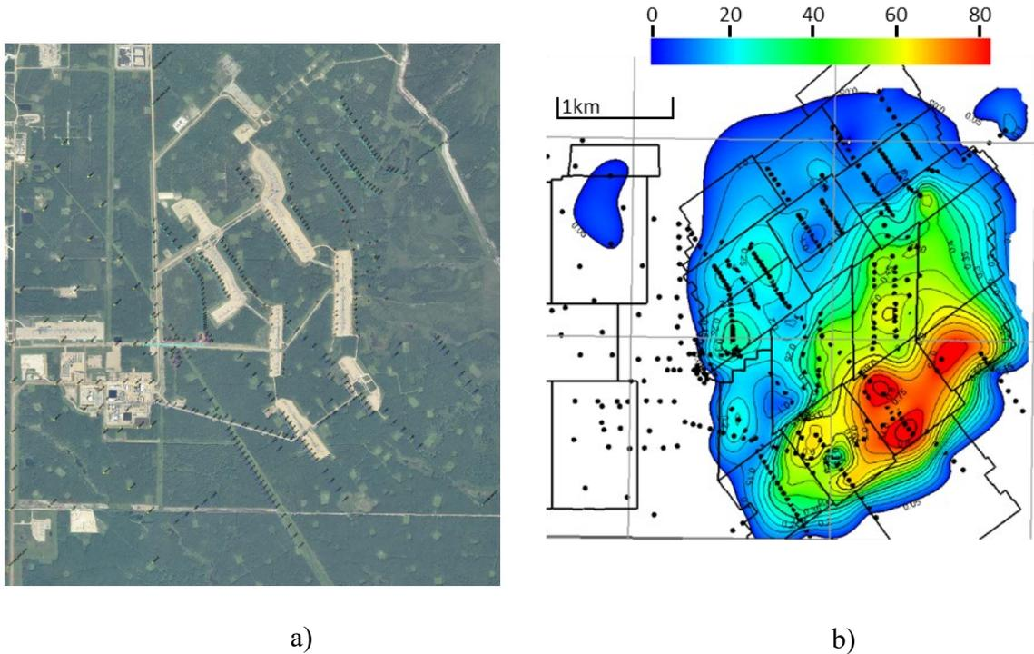
Figure 2-11 Surface heave monitoring at Suncor's MacKay River Project using survey monuments. a) aerial picture of MacKay River Suncor project. b) Surface heave obtained from surveys—originally published in Suncor Energy Inc. (2019b)
