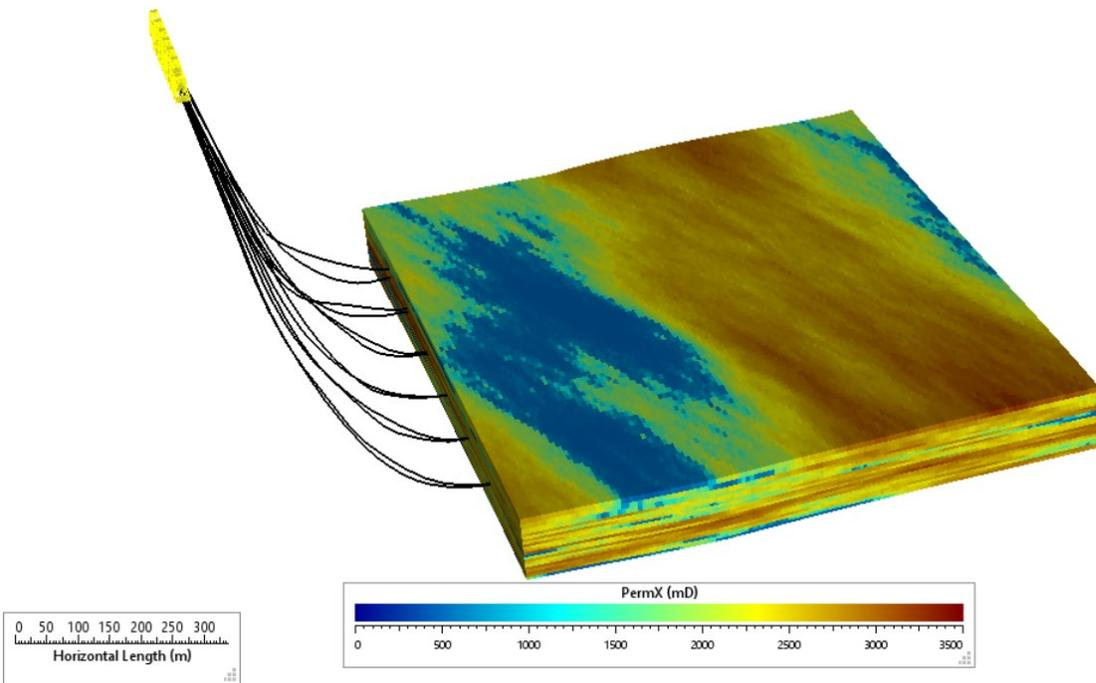
Figure 4-16 Horizontal permeability distribution of flow model for Pad AE.
