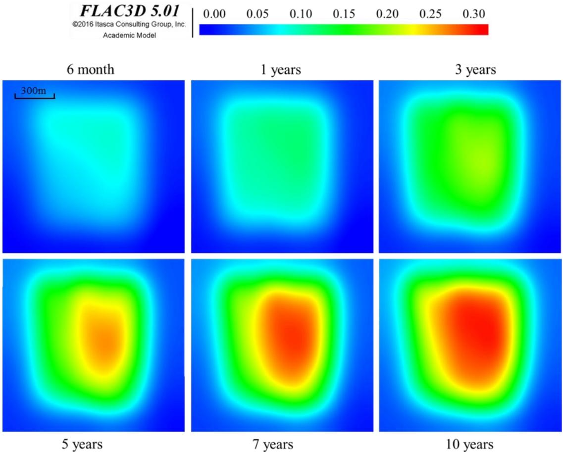
Figure 5-20 Predicted ground surface deformation in meters during SAGD operations below MOP
