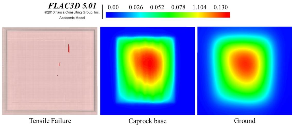
Figure 5-27 Tensile failure at the base of the caprock and vertical displacement at caprock base and ground surface.
