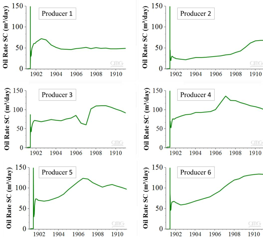
Figure 5-30 Oil rate production from all producer wells of the pad
