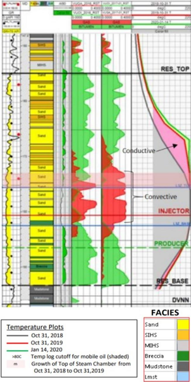
Figure 2-8 Typical temperature and saturations profile for Athabasca oil sands at three different times for Hangingstone Project, obtained from AER D54 2020 11888
