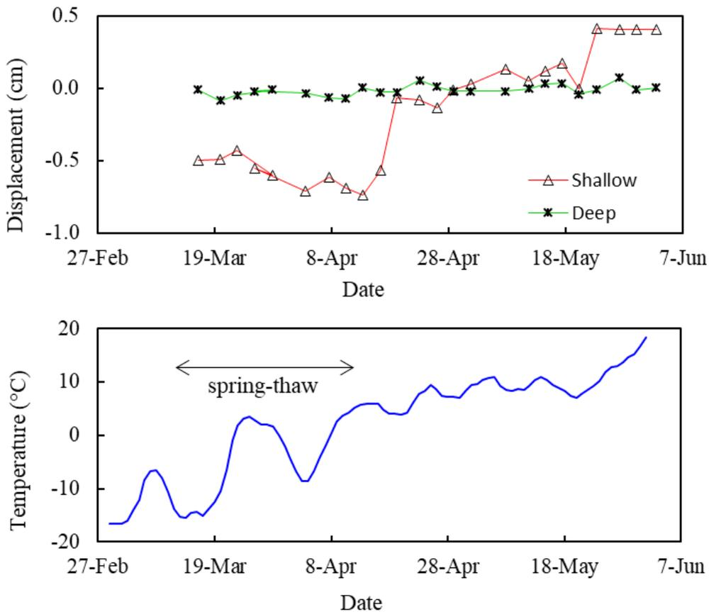
Figure 7-2 Impact of weather on corner reflector measurements.
