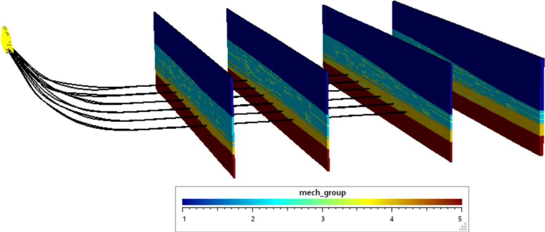
Figure 4-15 Geomechanical groups in Pad AE model at different cross-sections
