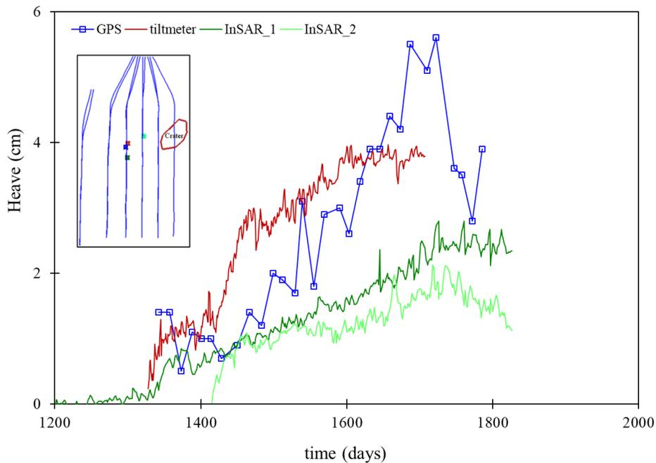
Figure 7-4 Comparison of measurements over time taken by different technologies located close to each other.
