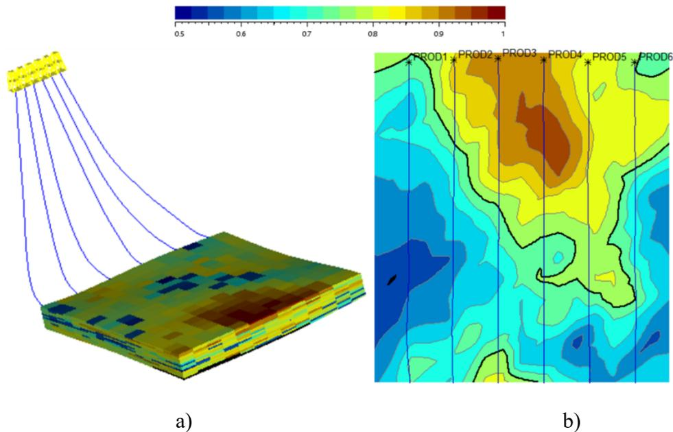
Figure 6-6 Reservoir Quality Index (CQI) for PAD AE at MRCP. a) 3D model of caprock with RQI for each cell. b) Aerial RQI map
