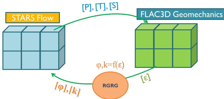
Figure 5-3 Sequential coupling simulation scheme (Deisman, 2017)
