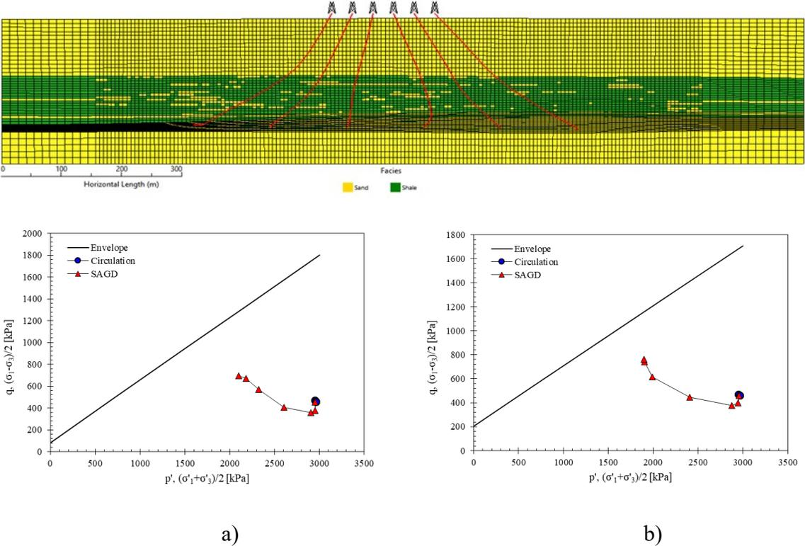
Figure 5-10 Stress path at two points in the middle of Pad in Clearwater formation. a) Silt in Clearwater b)Shale in Clearwater
