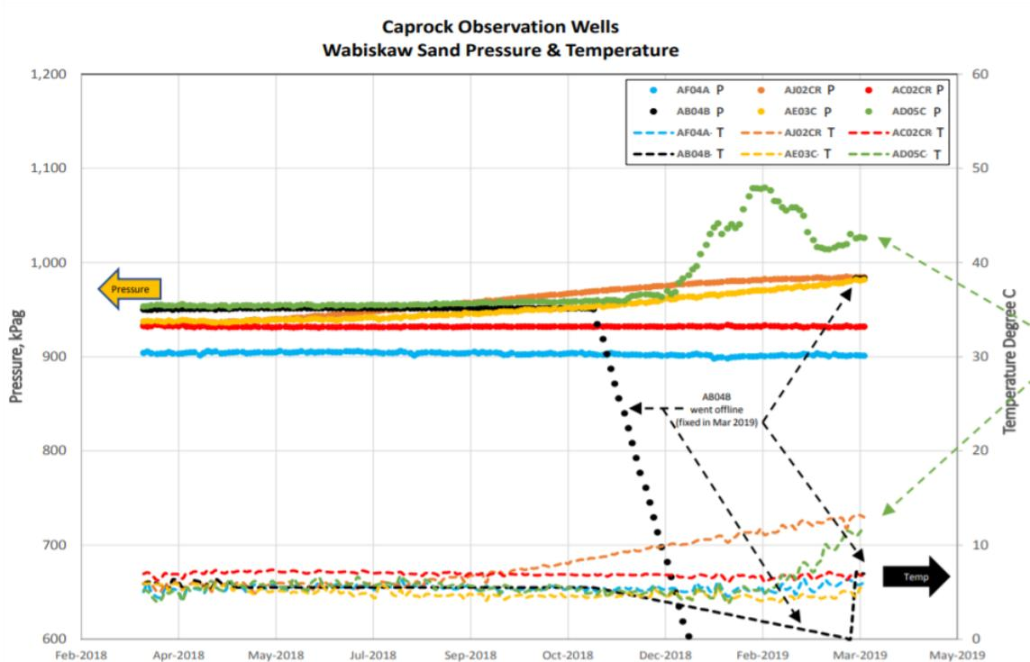
Figure 2-9 Temperature and pressure behaviour over time at Wabiskaw sand formation in PetroChina Canada's MacKay River project—originally published in PetroChina Canada (2019)
