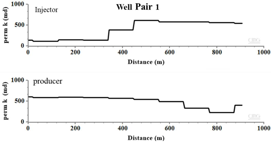
Figure 5-8 vertical permeability of blocks intersected by Well-pair 1.
