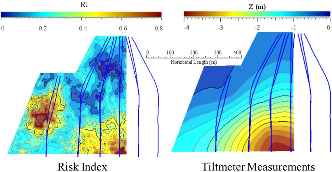
Figure 7-11 Surface deformation using tiltmeters selected from Risk Index calculation
