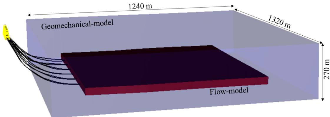
Figure 4-7 Flow model and Geomechanical model for Pad AE in MRCP.
