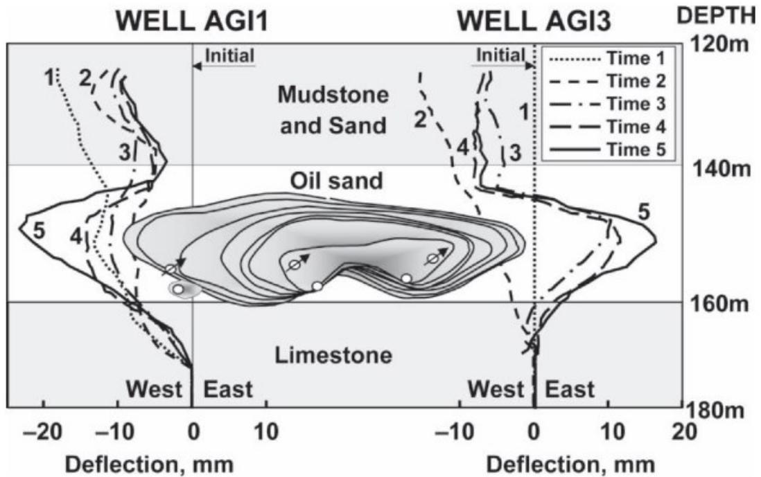
Figure 2-10 Horizontal displacements measured at UTF Phase A—originally published in Collins (1994)
