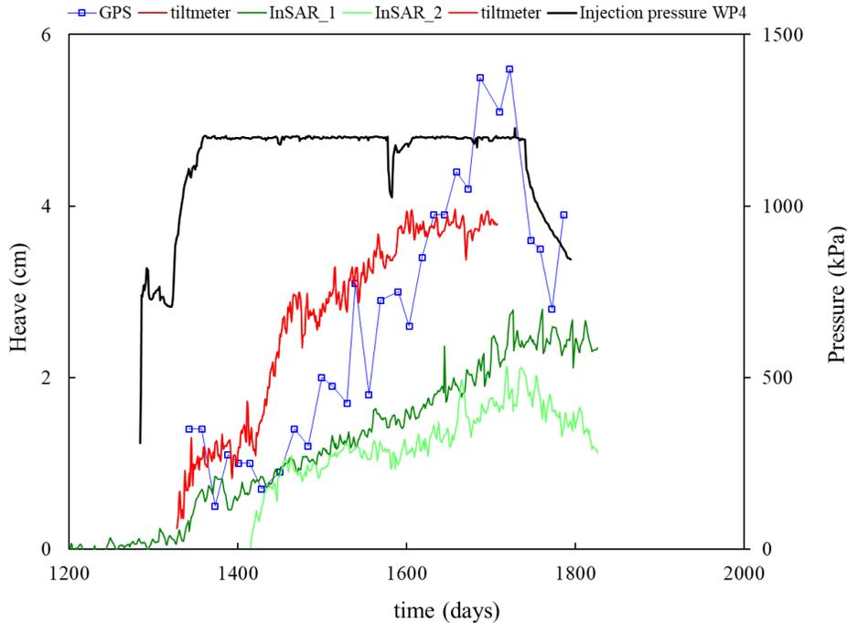
Figure 7-5 Injection pressure variation and surface heave observations from different monitoring techniques
