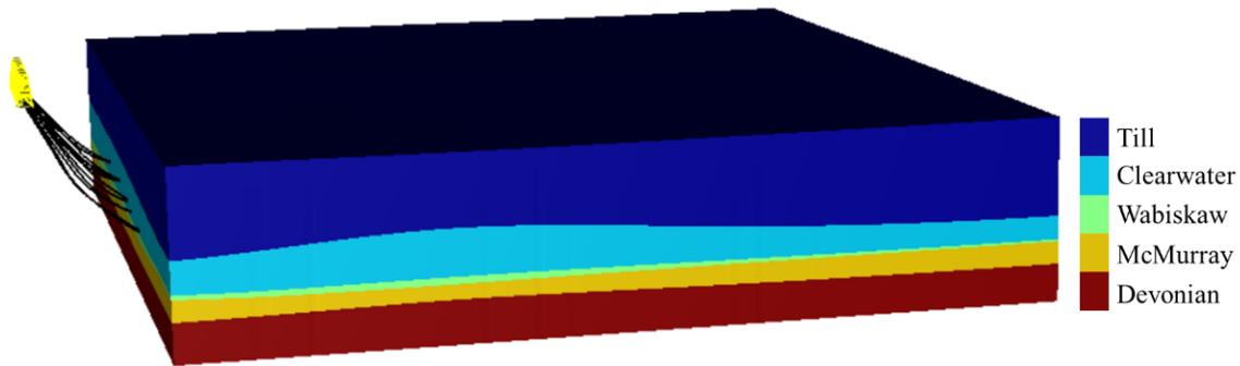
Figure 4-5 Layers constructed from horizons in the geomodel
