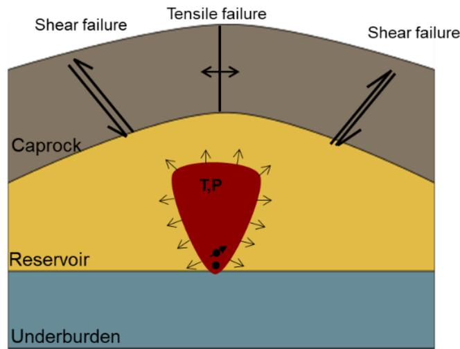
Figure 1-2 Schematic of possible failure mechanisms in the caprock during SAGD
