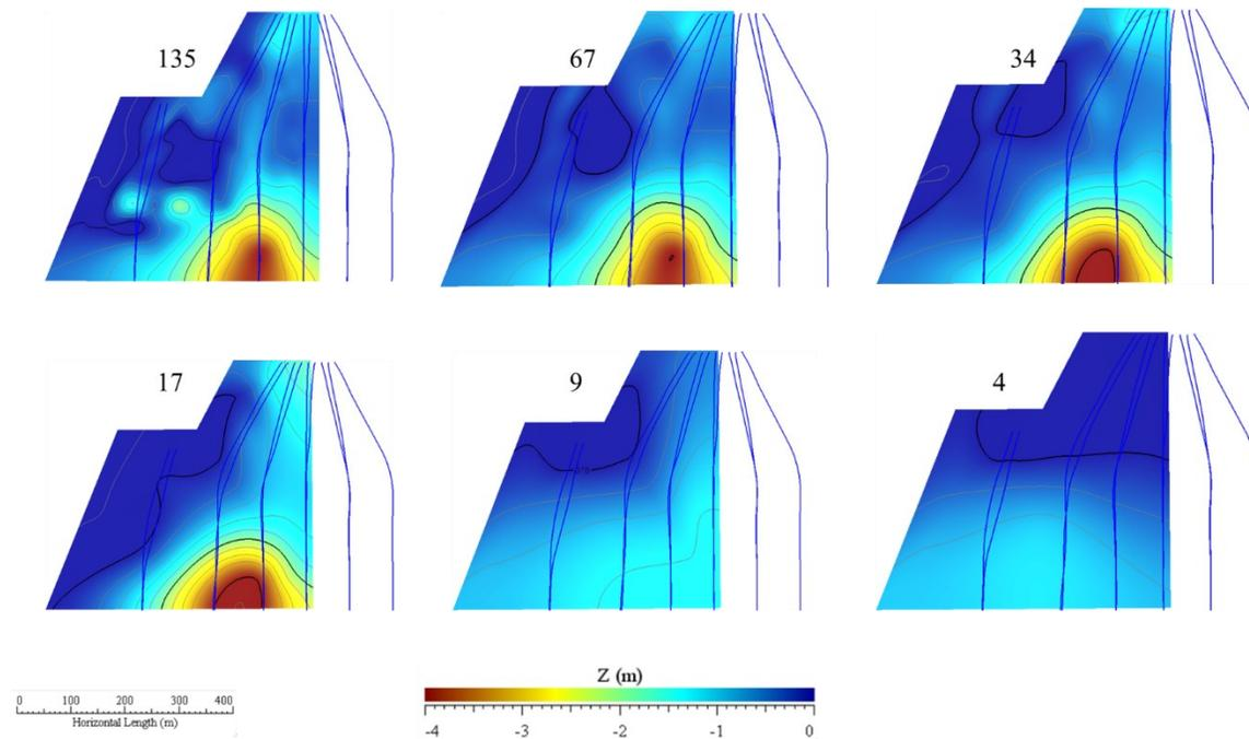
Figure 7-7 Vertical displacements contours from reduced tiltmeters
