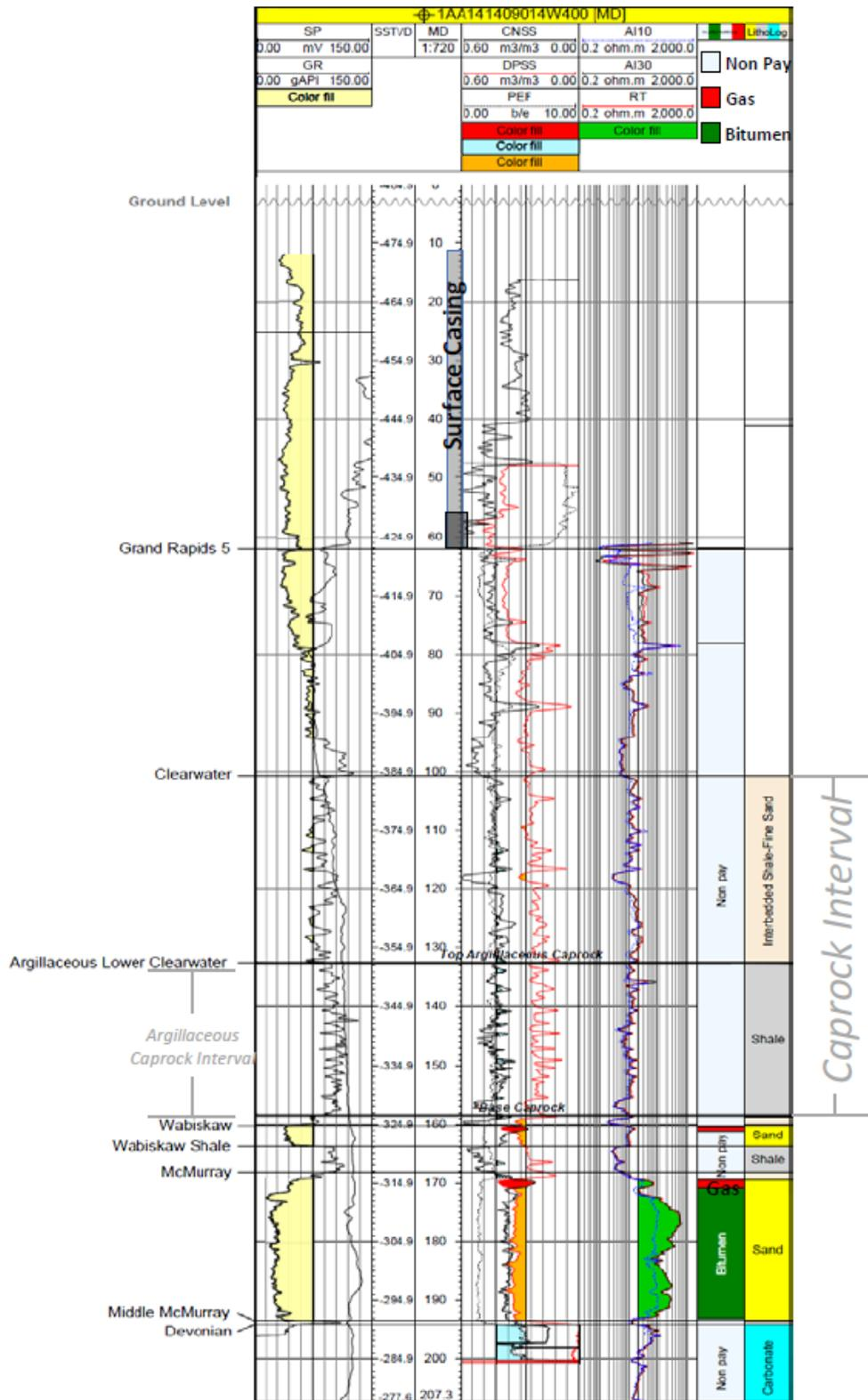
Figure 4-3 Typical stratigraphy and well logs in MacKay River Commercial Project area.
