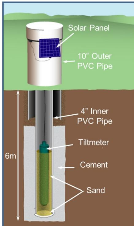
Figure 2-14 Scheme of tiltmeter installation
