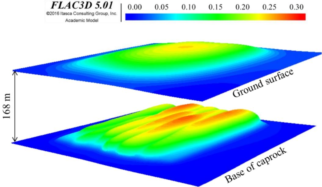
Figure 5-19 Predicted vertical displacement at the base of the caprock and ground surface after 4 years of SAGD
