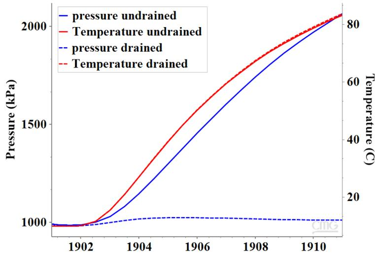
Figure 5-16 Simulated pressure and temperature at Wabiskaw Sand monitoring zone for drained and undrained conditions.
