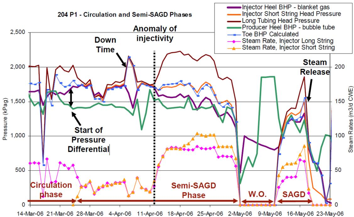
Figure 2-15 BHP and flow rate behaviour on injection well at Joslyn's steam release location—originally published in Energy Resources Conservation Board (2010)
