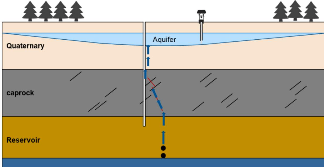
Figure 1-3 Different pathways that can be generated or opened during steam injection, allowing flow from the reservoir to the upper layers.
