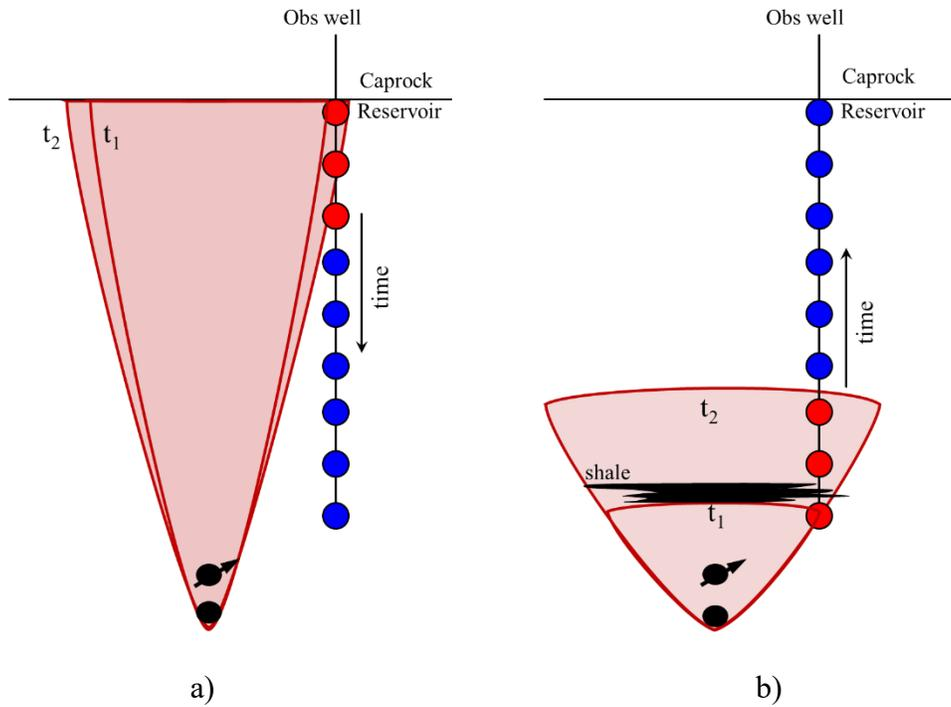
Figure 5-13 Temperature readings behavior at observation wells for a) homogeneous reservoir.
