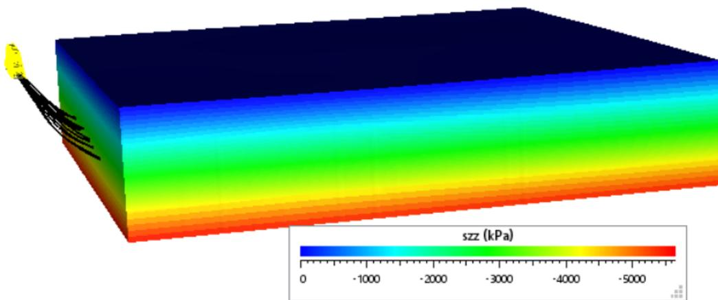
Figure 4-13 Calculated vertical stress at Pad AE model.
