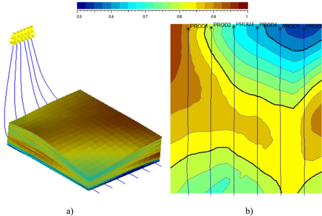
Figure 6-5 Caprock Quality Index (CQI) for PAD AE at MRCP. a) 3D model of caprock with CQI for each cell. b) Aerial CQI map.
