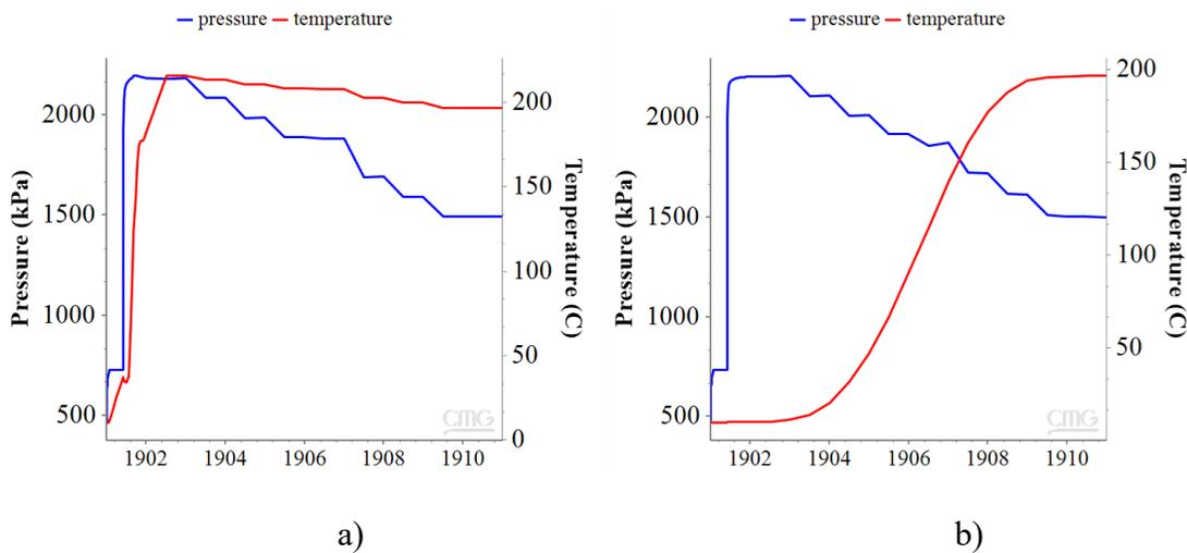
Figure 5-15 Pressure and temperature behavior at two different locations within the reservoir. **a)** a few meters away from a well-pair. **b)** At the middle of two well-pairs.
