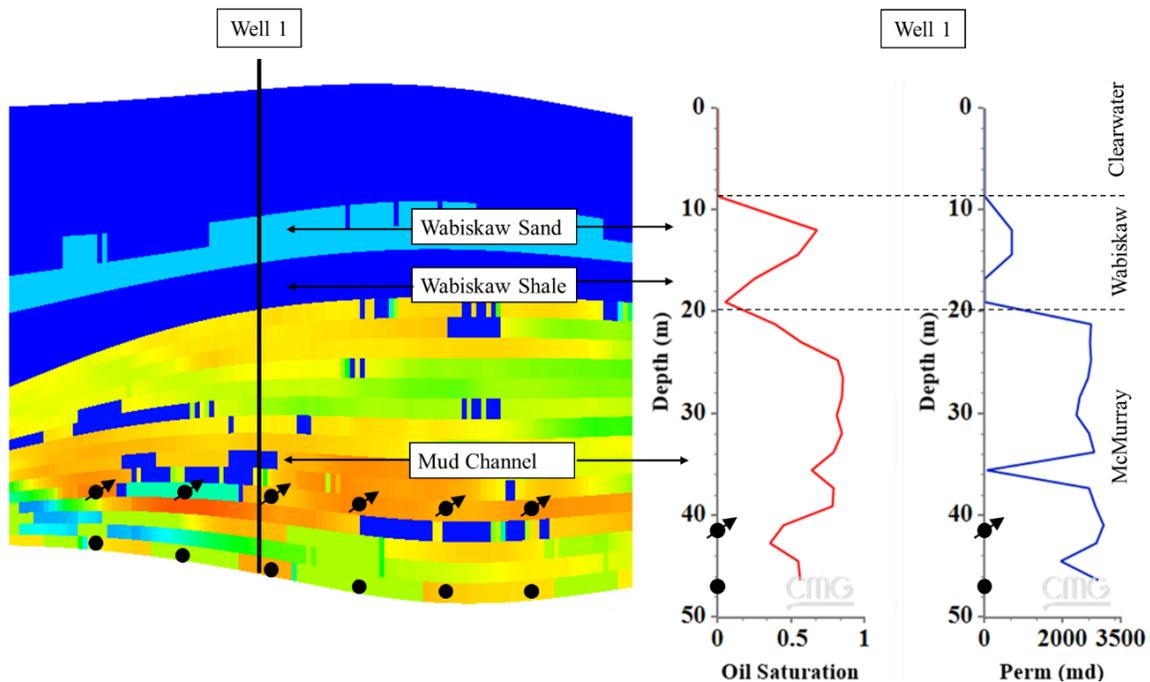
Figure 5-11 Permeability heterogeneity of a 2D cross-section for a heterogeneous model and the oil saturation and permeability profile at Well 1.
