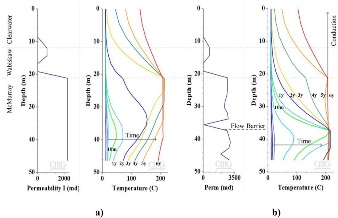
Figure 5-12 Predicted temperature profile at Well 1 for: a) homogeneous model and b) heterogeneous model
