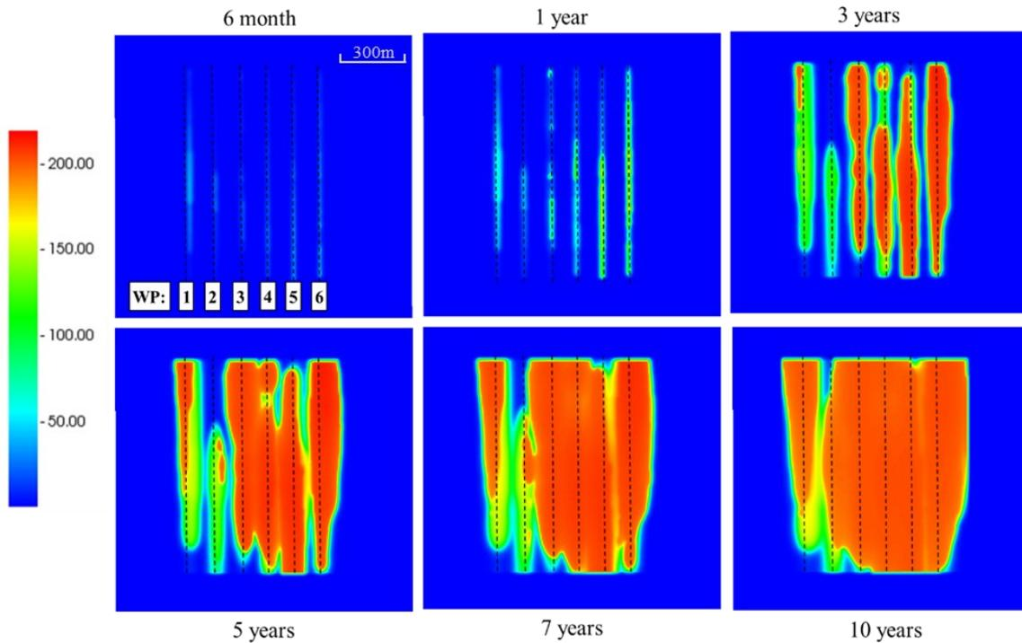
Figure 5-22 temperature distribution at the top of the reservoir during SAGD below MOP
