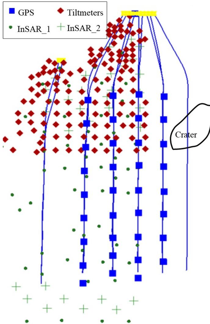
Figure 7-1 Heave monitoring instruments at Pad 204 Joslyn's SAGD Project after the 2006 blowout
