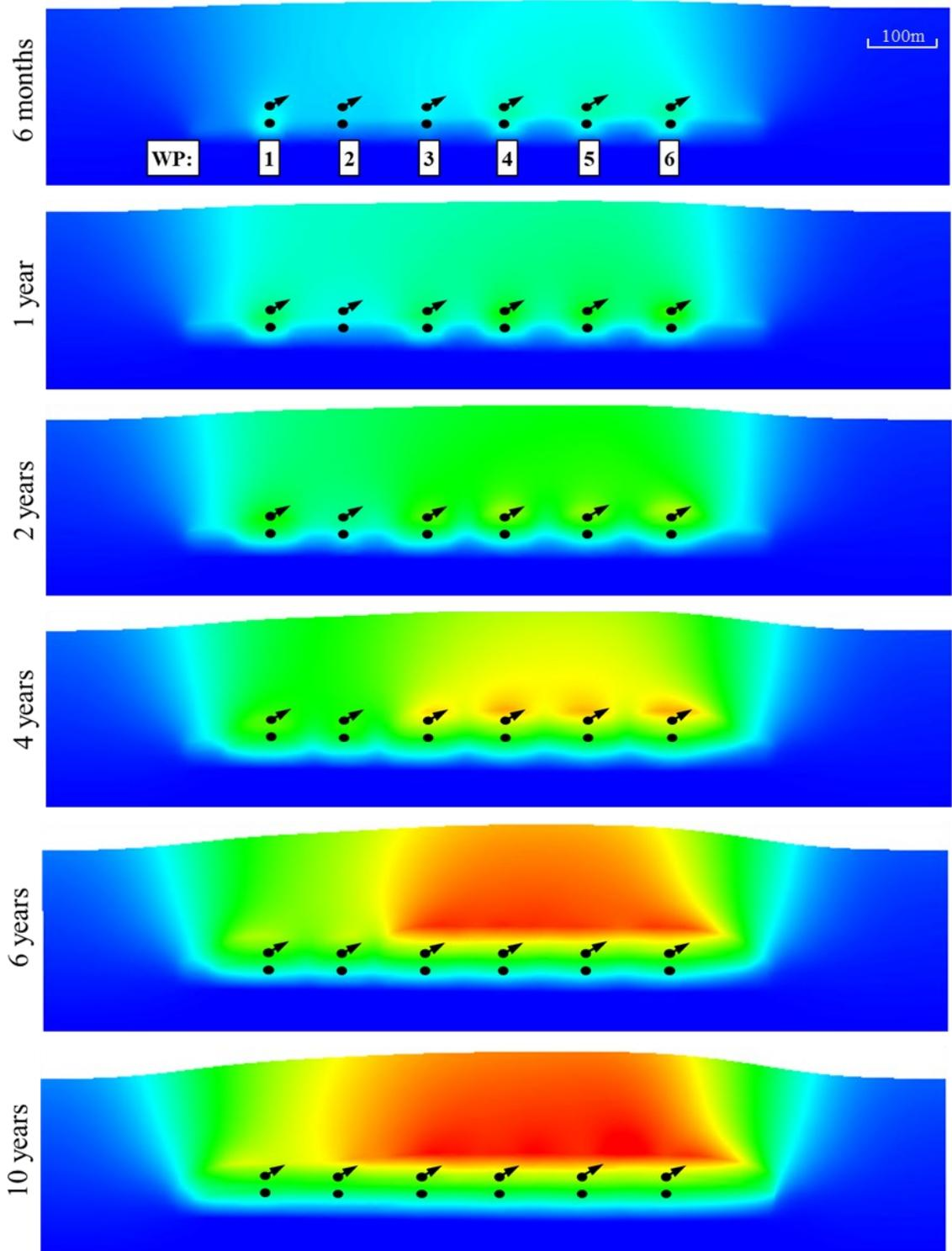
Figure 5-23 2D cross-section of simulated vertical displacement perpendicular to the well-pairs
