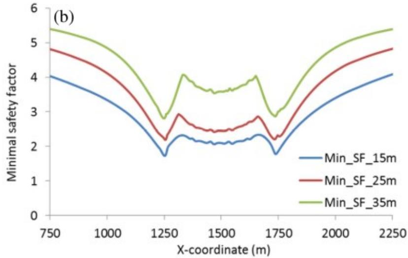
Figure 6-1 Impact of caprock thickness on the safety factor in SAGD. Taken from (Xiong & Chalaturnyk, 2015)
