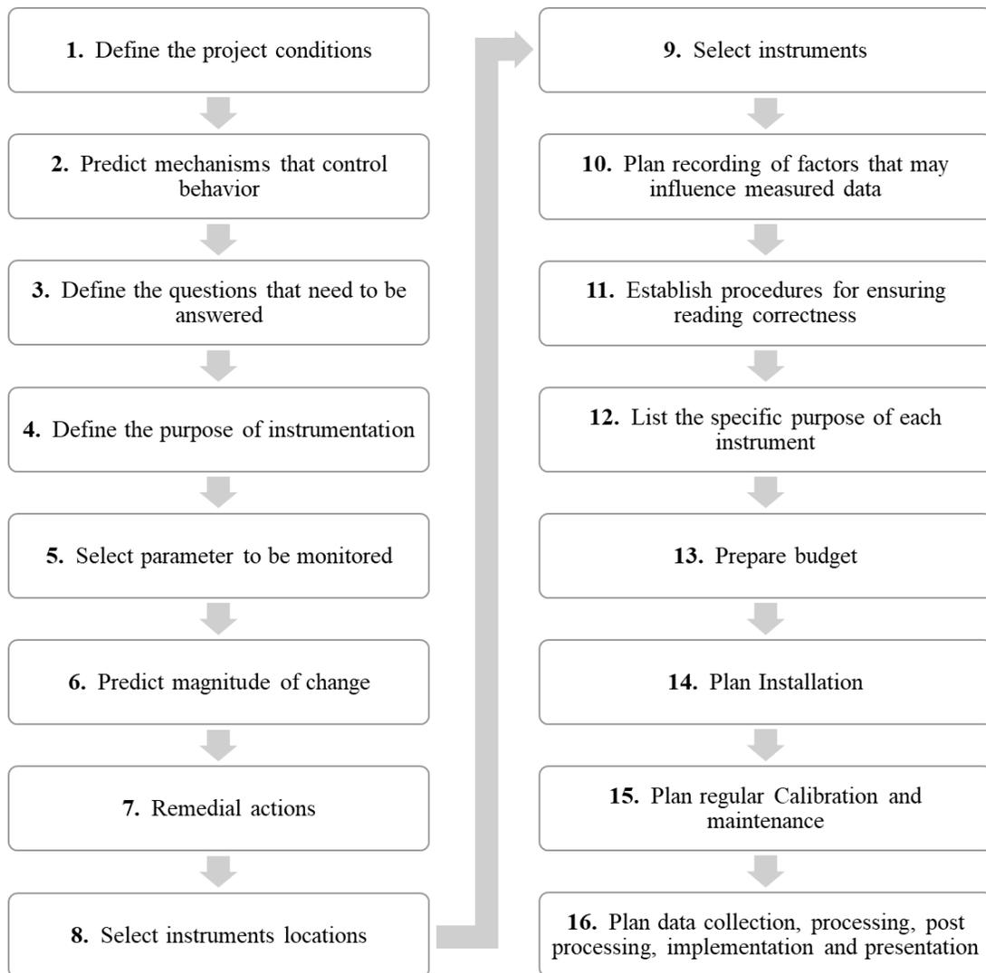
Figure 3-1 Workflow for systematic approach to designing geotechnical monitoring as proposed by Dunnicliff (Modified from Dunnicliff, 1988)
