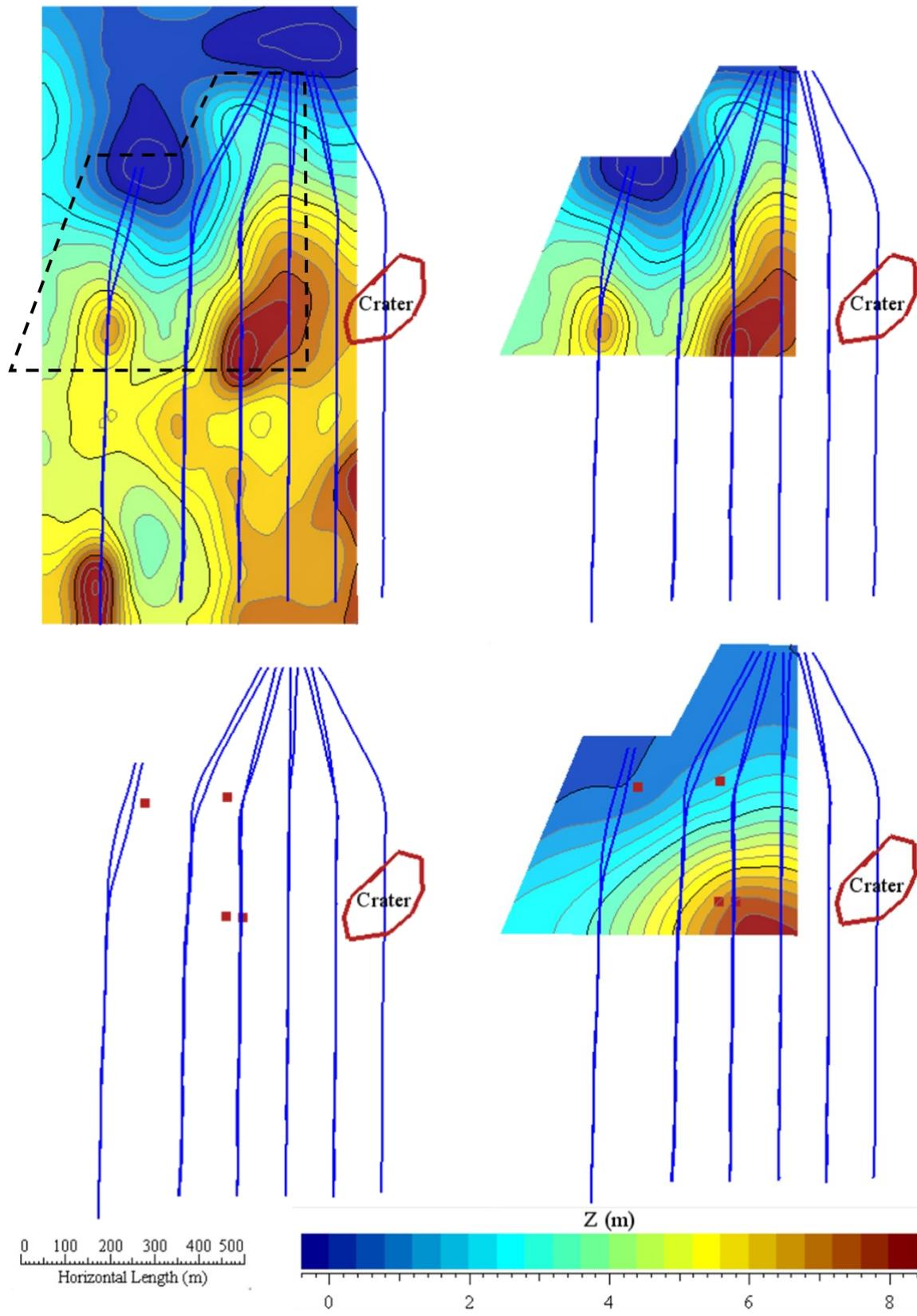
Figure 7-10 Surface deformation using tiltmeters selected from numerical simulation results
