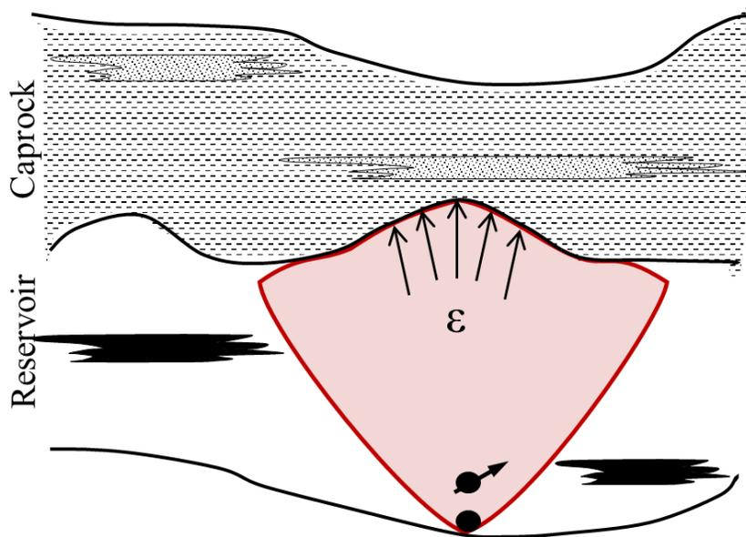
Figure 6-2 Schematic of conditions to initiate fracture in the caprock
