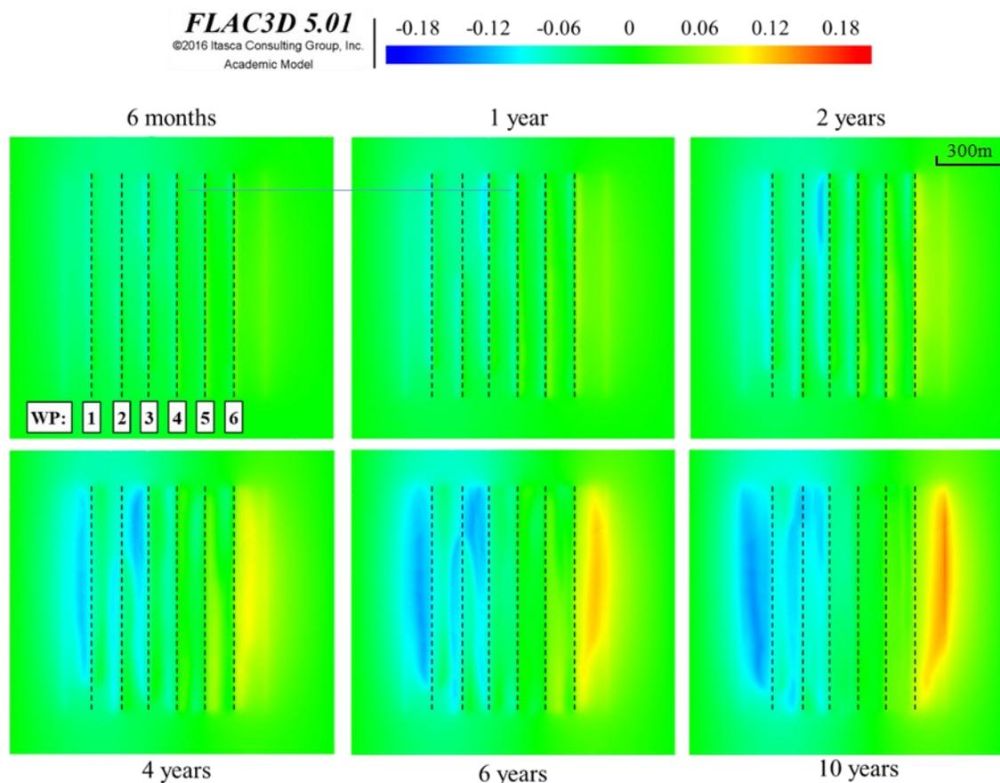
Figure 5-18 Horizontal displacements at injectors' depth for different times.
