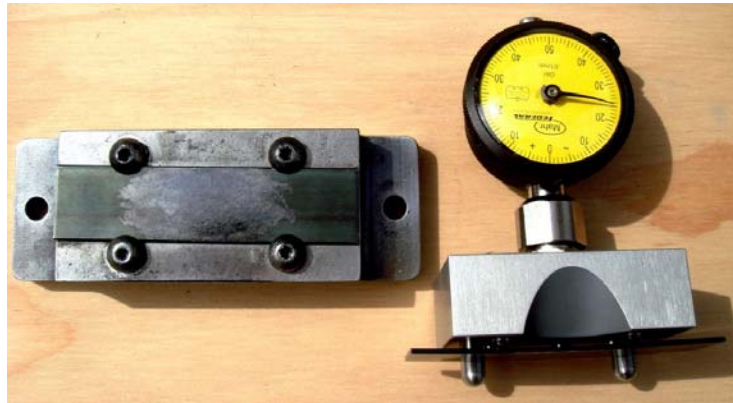
Figure 5.3 – Almen strips, holder and gauge.
