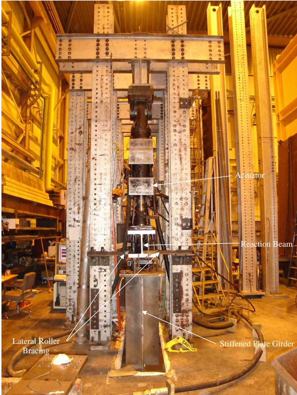
Figure 5.13 – End view of large scale test set-up.
