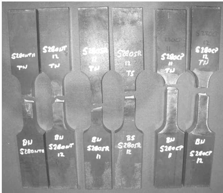
Figure 5.9 – Failed small scale specimens with as-is weld profile.
