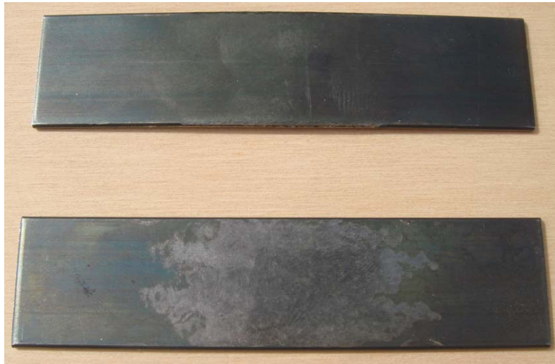
Figure 5.5 – Impacted surfaces of conventionally (top) and ultrasonically (bottom) peened Almen A-strip.
