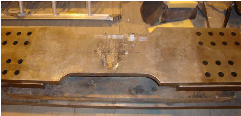
Figure 5.22 – Typical “dog bone” plate.
