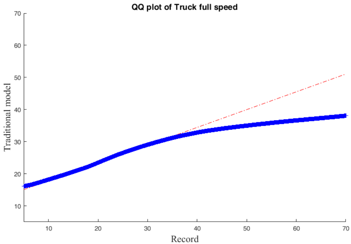
Figure 4.18 QQ plot of truck full speed of the traditional simulation model and real operational records
