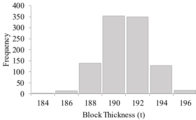
Fig. B-17 Block Thickness (Normal Distribution)
