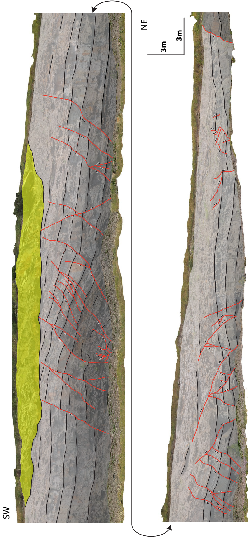
Figure 3.13. Interpreted orthomosaic photo of the Highway 1 roadcut.
