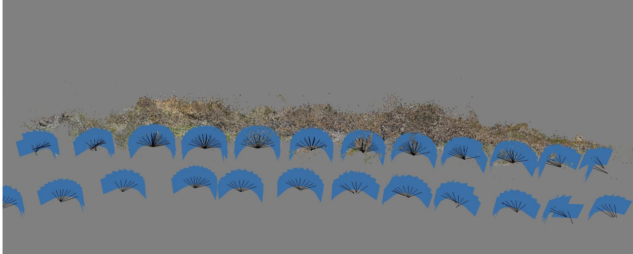
Figure 2.7. A screen capture from AgiSoft Photoscan Professional showing the aligned cameras.
