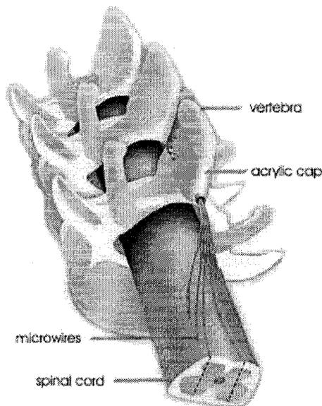
Figure 1.1: Example of ISMS implant. The exposed spinal cord is implanted with microwires deinsulated only at the tips. The microwires are Pt-Ir (platinum-iridium) or stainless steel with diameters of 25-30  $\mu$ meters. Stimulation through these wires, implanted to target the ventral horn, has been shown to produce multi-joint synergies and functional weight bearing stepping (see text).
