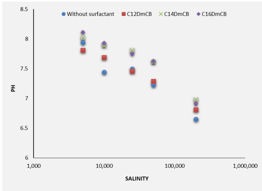
Figure 5. 4 The pH of the brine/limestone system with salinity in SFW and various C n DmCB surfactant solutions
