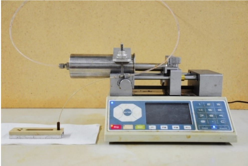
Figure 6. 1 The experimental setup of the micromodel flood test
