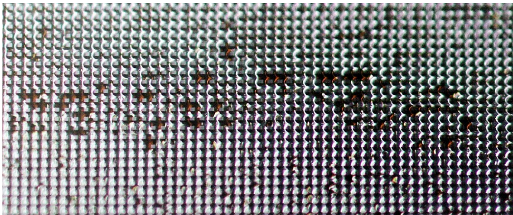
Figure 6. 5 Residual oil trapped in the water-wet pore structures
