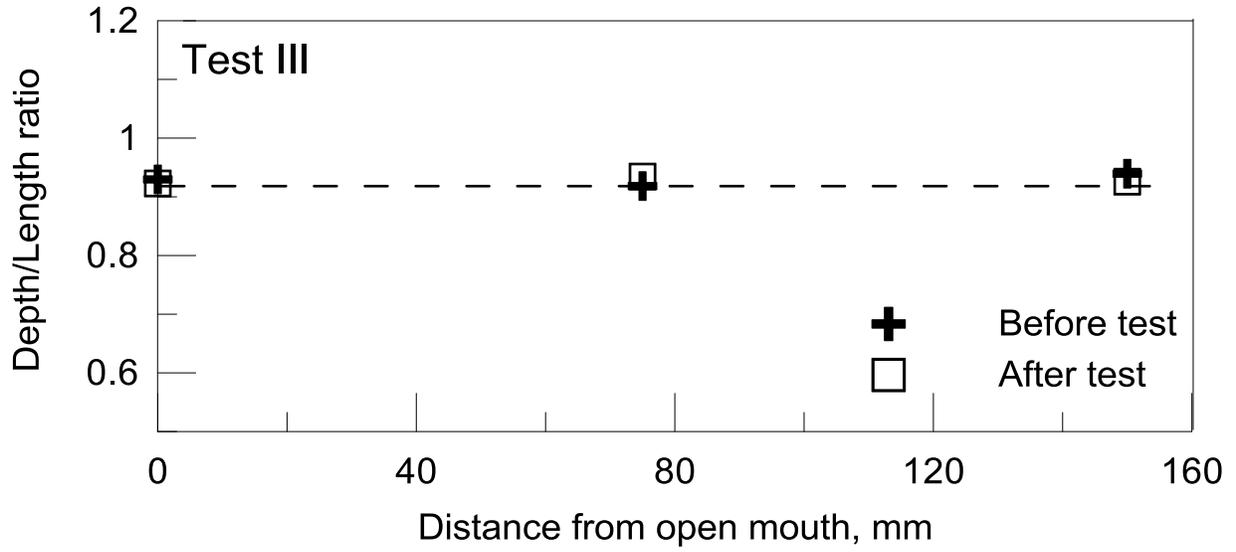
Figure 4-17: Aspect ratios of cracks in Test III
