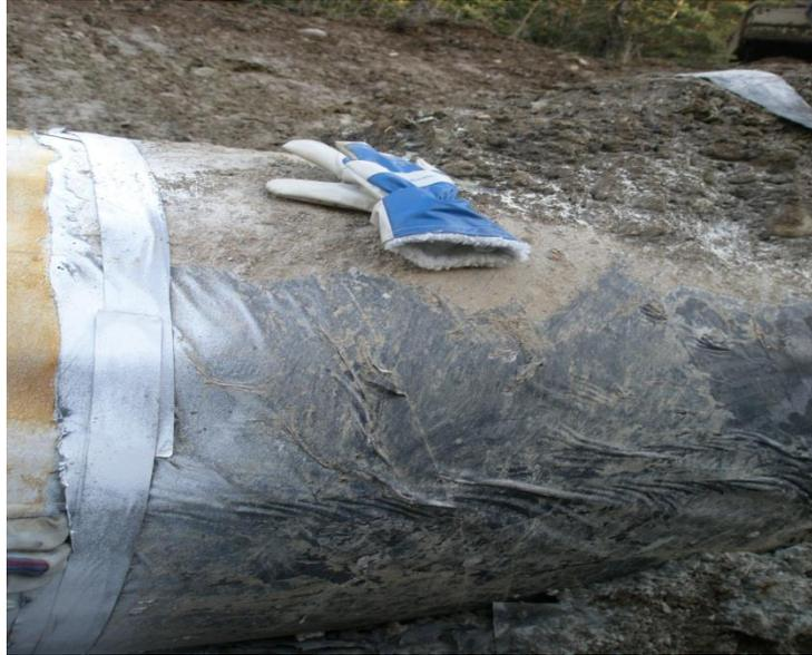
Figure 2.9: showing a pipeline in which severe de-bonding of the polyethylene coating has occurred.
