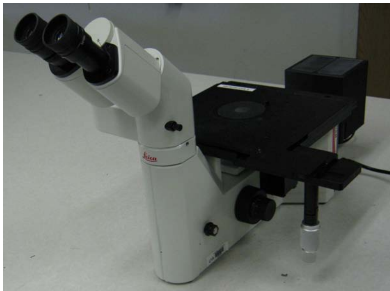
Fig. 2-4. Leica microscope for observing wear tracks
