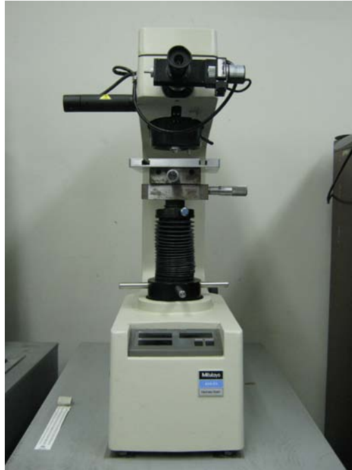
Fig. 2-6. Mitutoyo AVK-C1 hardness tester
