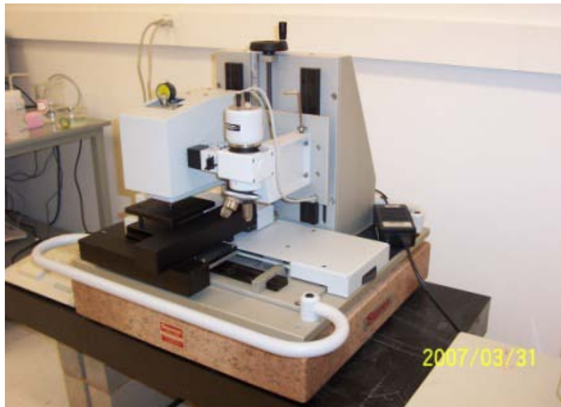
Fig. 2-8. A micro-indentation system (Fischerscope H100C)
