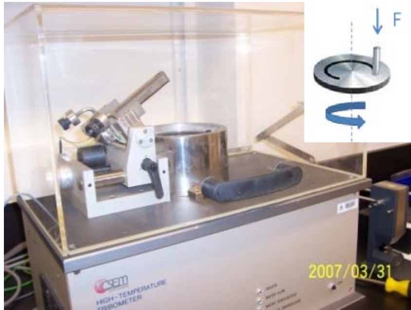
Fig. 2-3 A pin-on-disc tester for the present wear tests
