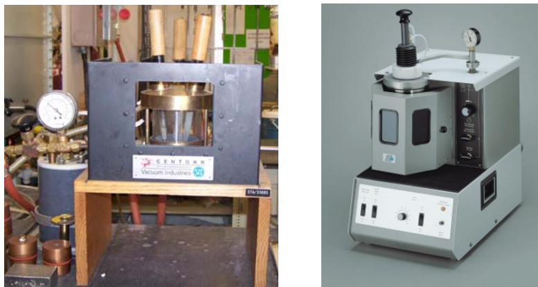
Figure 1–10. The arc melters in our lab used for the arc-melting: (a) Centorr 5TA tri-arc melter; (b) Edmund Bühler arc melter.
