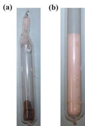
Figure 1–11. The reaction tubes for direct reaction: (a) fused silica tube; (b) alumina tube.
